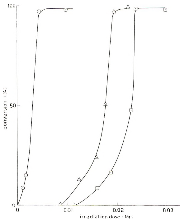
Fig. 1. In-source polymerization of glass-forming systems containing acrylamide and acrylic acid: (○) acrylamide-propionic acid-formamide (1.1:0.5); (△) acrylic acid-acetamide (1:0.5); (◻) acrylic acid-formamide (1:1). Temperature, -78^{\circ}\text{C} .; dose rate: 1.5 \times 10^4 r./hr.
