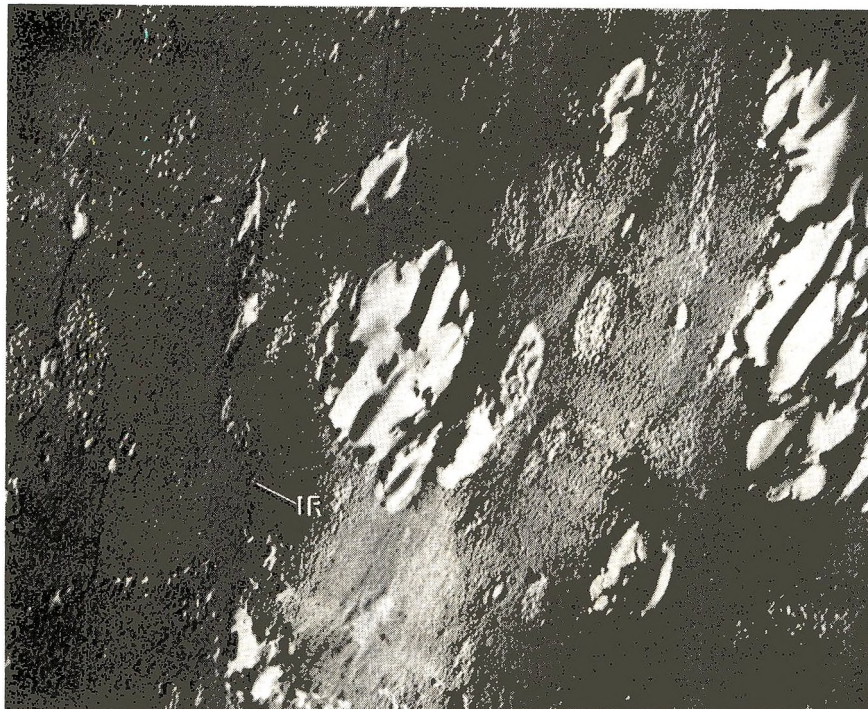
Fig. 9. Electron micrograph of wool grafted about 2800%, shadowed at \tan^{-1} 0.8 ( \times 18,000 ).
