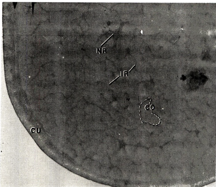
Fig. 2. Electron micrograph of cross section of unstained native wool ( \times 24,750 ). The following nomenclature is used in this and subsequent micrographs: IR, intercellular regions, NR, nuclear remnants, CU, cuticle, CO, cortical cell, EM, embedding medium, H, homopolymer.
