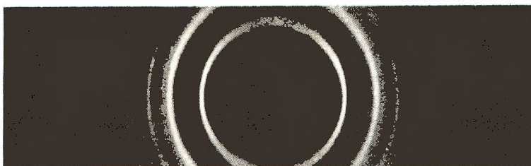
Fig. 1. Polyvinylcyclopropane powder, heptane-insoluble fraction, heat-treated \frac{1}{2} hr at 175–180°C. Powder camera, 114.6 mm diameter.
