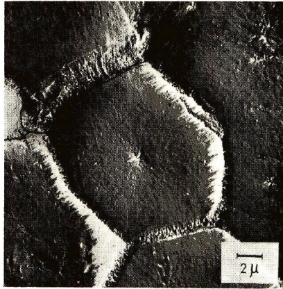
Fig. 2. Electron micrograph of film 1 stretched polyaxially at 130°C in poly(ethylene glycol); v_A = 1.4 .
