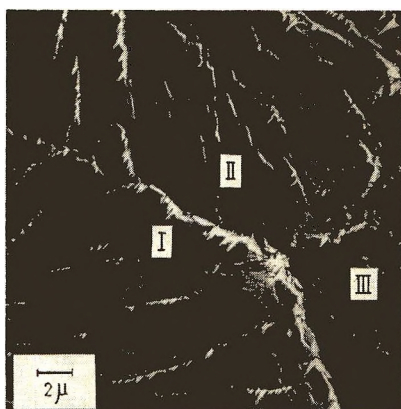
Fig. 9. Boundaries between three spherulites, I, II, and III of film 5 stretched biaxially at 140°C in air; v_A = 1.2 . Breaking can be seen between the boundaries (I,II) and (I,III) but not at the boundary (II,III). Also cracking occurs radially on I and II but tangentially on III.
