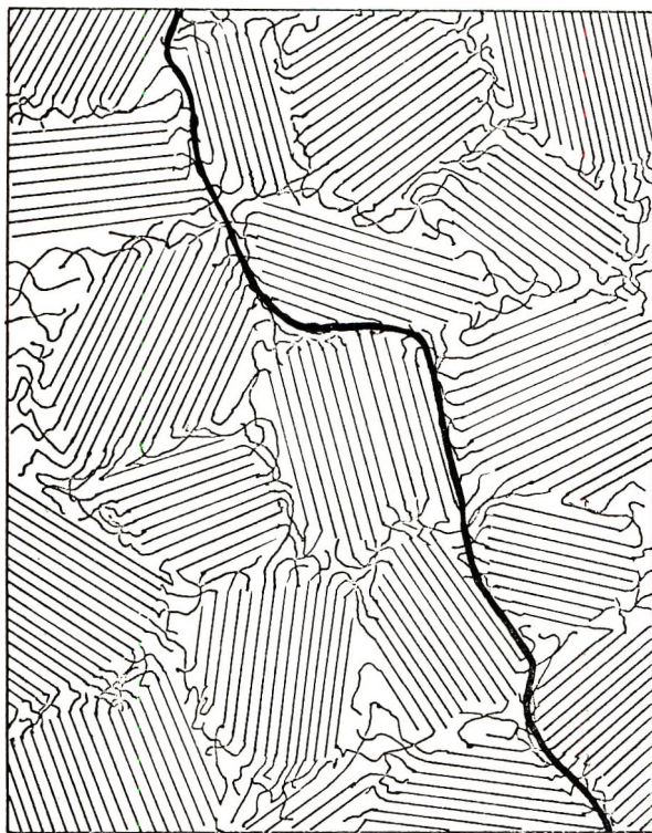
Fig. 8. Flory's fringed micelle model of a semicrystalline polymer showing a selective fracture path.
