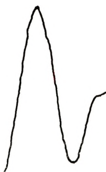
Fig. 9. Very weak EPR spectrum from several pieces of PMMA after fracture.
