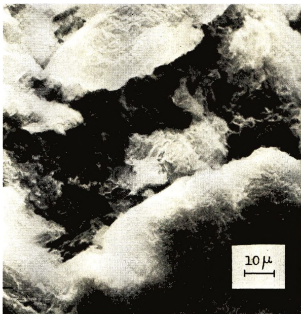
Fig. 4. Scanning-type electron micrograph of the crystalline aggregate of polyoxymethylene formed by the polymerization of trioxane in nitrobenzene.
