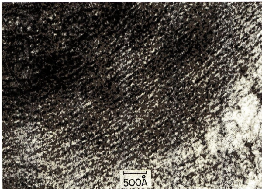
Fig. 6. A higher-resolution electron micrograph of thin cross section of the 101.6% grafted sample showing appearances of the layers in outer region of a macrofibril. A large amount of polymer deposition can be seen on the right side.
