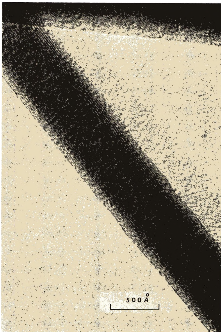
Fig. 10. Lattice image of a chrysotile polymer fiber in a horizontal position.
