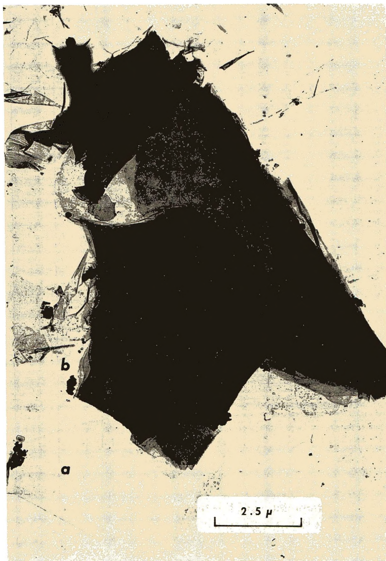
Fig. 13. Bent ( a ) and stacked ( b ) sheets of the apophyllite polymer.
