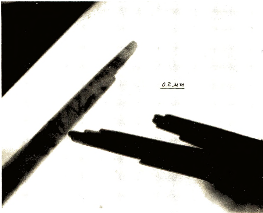
Fig. 4. Electron photomicrograph of 3T nylon crystals at high magnification.
