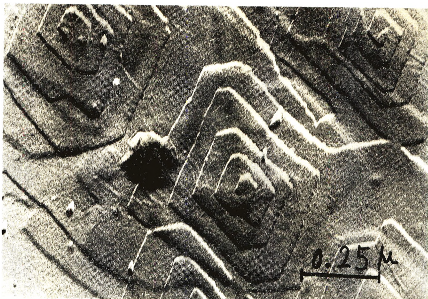
Fig. 8. Well defined crystals of 2-8 polyester formed through spiral growth on the mother crystal. Note that the dimensions of such well-defined crystals are very small, ( \leq 0.5 \mu ).
