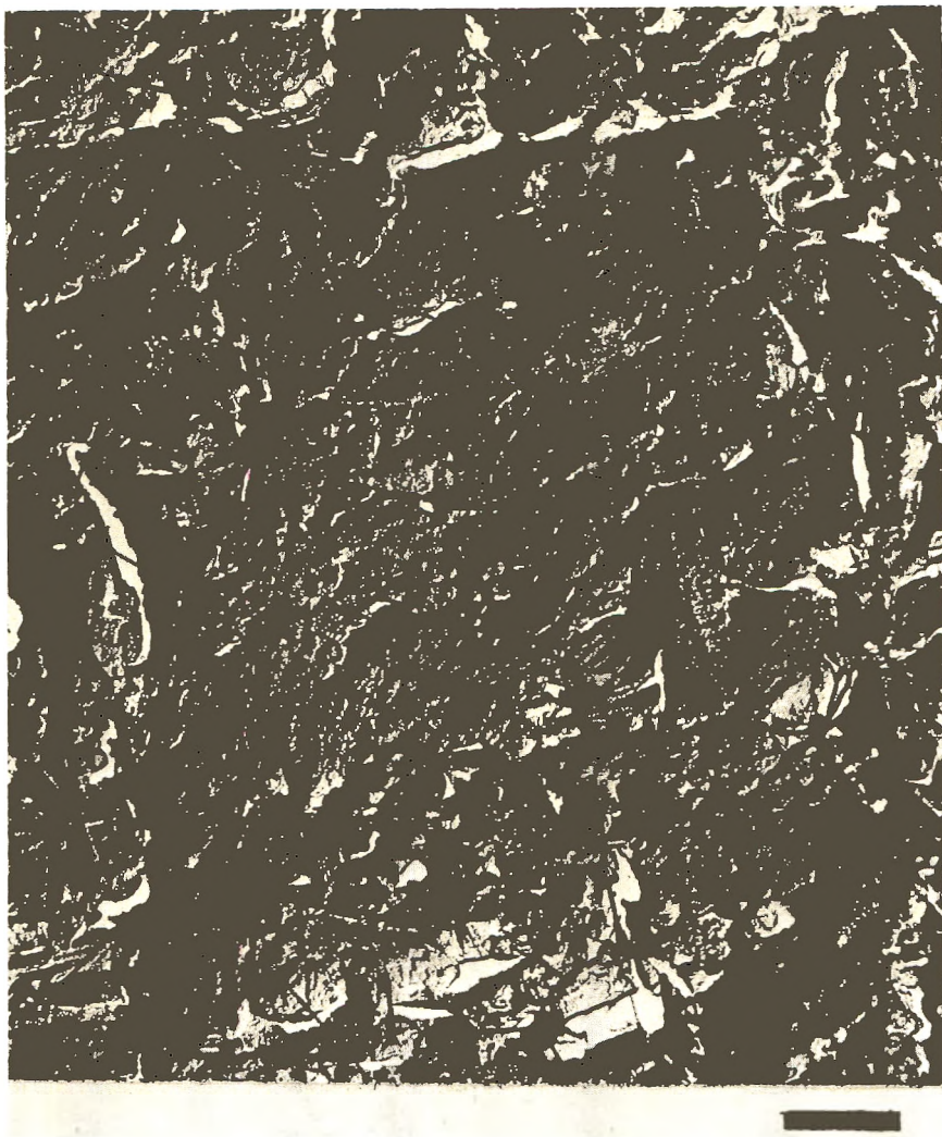
Fig. 6. Drawn fracture surface from a mixture containing 75 w% HMW material crystallized at 2000 atm. Only a few thin, extended-chain lamellae are visible (center right). The scale bar designates 1\mu .
