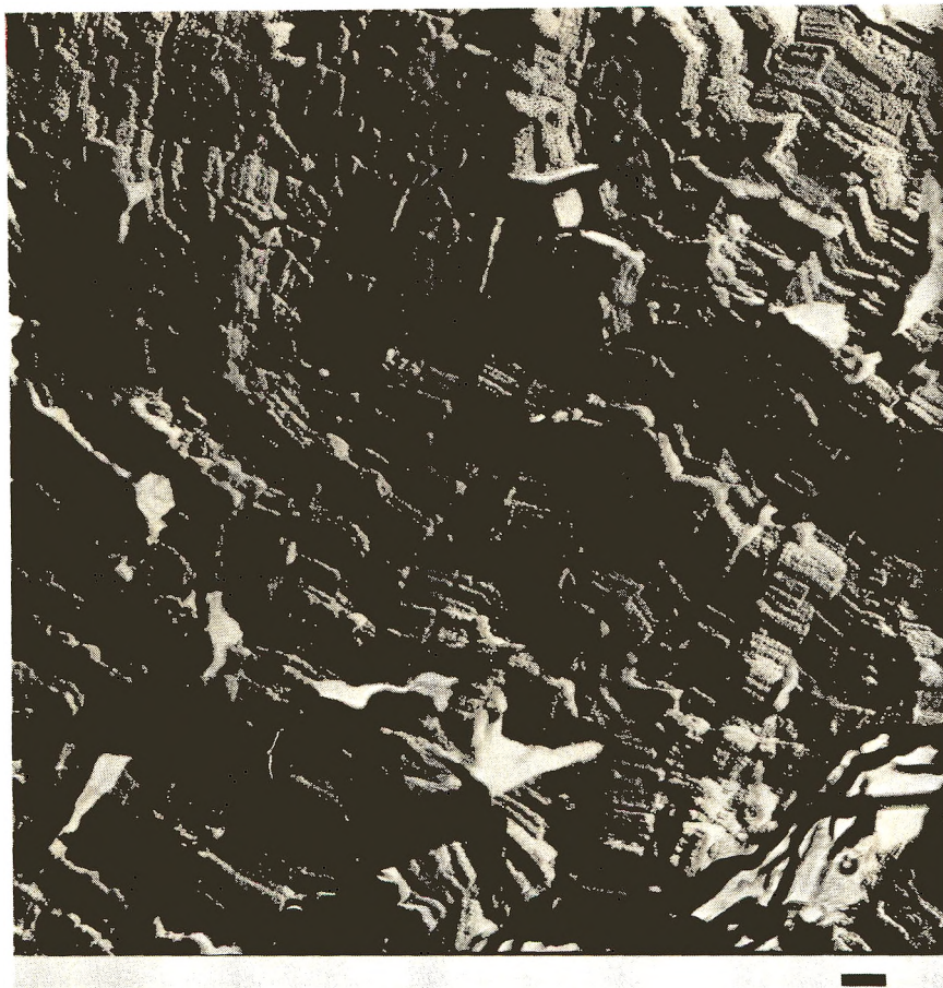
Fig. 8. High magnification view of a portion of Figure 7 showing many thin extended-chain lamellae which have crystallized nearly parallel. The scale bar designates 0.1 \mu .
