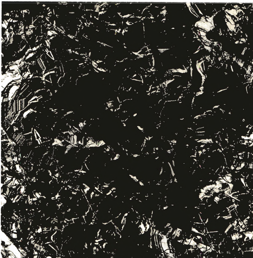
Fig. 3. Fracture surface from HMW fraction of linear polyethylene crystallized at 3000 atm. Note the dark fibrils indicative of folded-chain or imperfectly crystallized material. Points of lamella termination and impingement are designated by arrows. The scale bar represents 1\mu .
