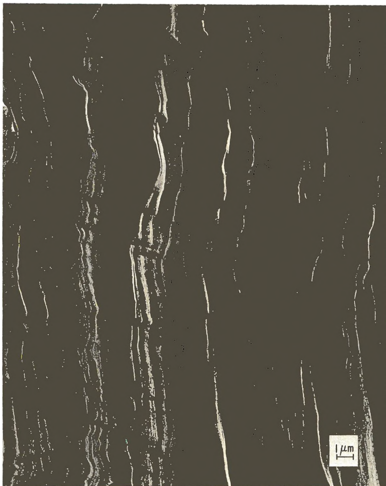
Fig. 3. Electron micrograph of a rippled surface; oriented high-density polyethylene, not annealed.
