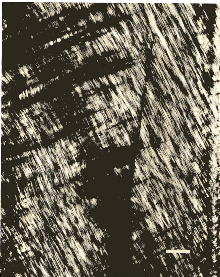
Fig. 6. A specimen containing both a rippled region and a kink band. This specimen had been sheared (right side upward, left side downward) 10% at the rate of approximately 10 \text{ min}^{-1} and then 20% at approximately 0.1 \text{ min}^{-1} . The marker represents 10 \mu .
