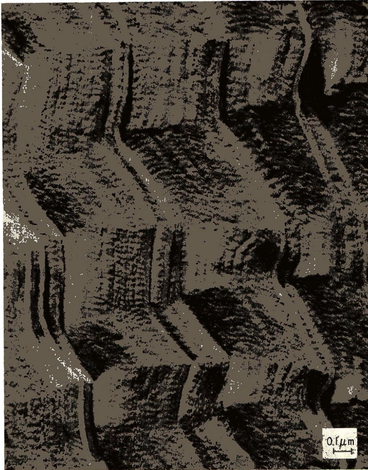
Fig. 4. Electron micrograph of a rippled surface after about twice the strain as that in Fig. 3; annealed, oriented high-density polyethylene.
