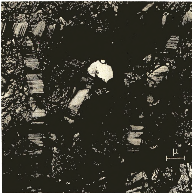
Fig. 8. Framework of thick lamellae in Marlex 6002 homopolymer crystallized at 232°C for 30 min.
