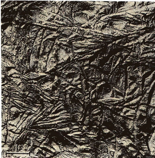
Fig. 6. Snaking lamellae in fraction C crystallized at 210°C for 30 min.
