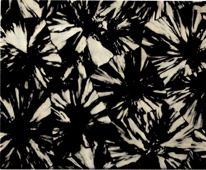
Fig. 11. "Mixed" nylon 97 positively birefringent spherulites with ringed centers (spacing 3.8 \mu ) which fan into an aggregatelike structure. Fusion temperature 254^{\circ}\text{C} (1/4 hr); crystallized 200^{\circ}\text{C} (16 hr). \times 400 .
