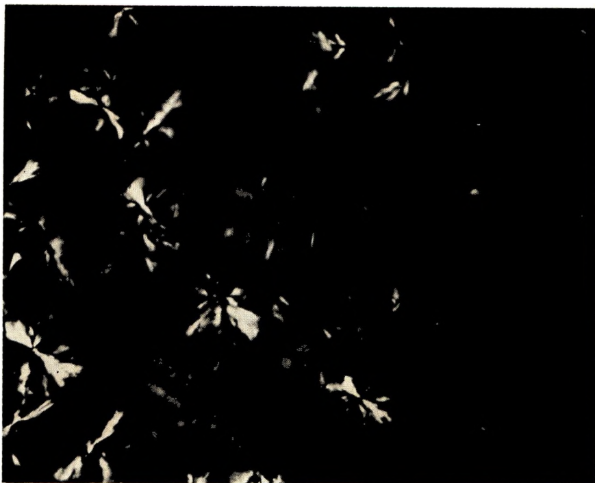
Fig. 5. Nylon 57 low-birefringent platelets and higher-birefringent aggregates formed at 215°C (3 hr); fusion temperature 230°C (1/2 hr). \times 415 .
