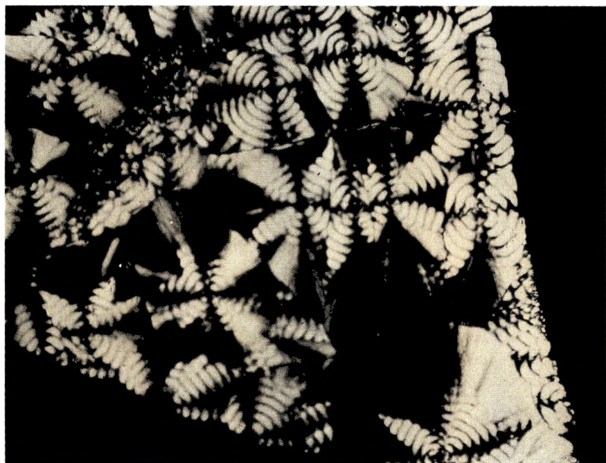
Fig. 6. Nylon 77 ringed negative spherulites ( 4.3 \mu spacing) with zigzag extinction cross formed at 187°C. Fibrillar overgrowths are also apparent. Fusion temperature was 260°C (1/2 hr). \times 790 .
