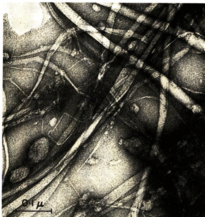
Fig. 3. Preparation of Valonia ventricosa as visualized by the negative staining technique in the absence of a supporting carbon film. The specimen is supported in a thin film of uranyl acetate suspended over a hole in a carbon film. Electron micrograph, magnification 157,000 \times .
