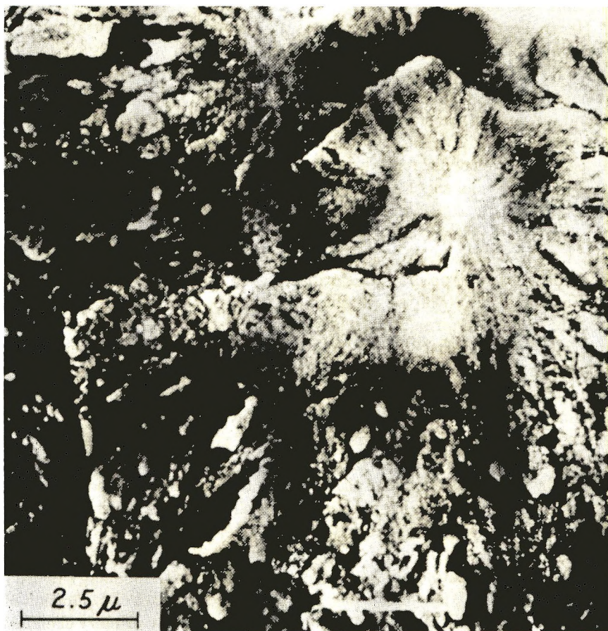
Fig. 17. Electron micrograph of poly(methyl methacrylate) after exposure to a laser beam with energy density of 10 joule/cm 2 .
