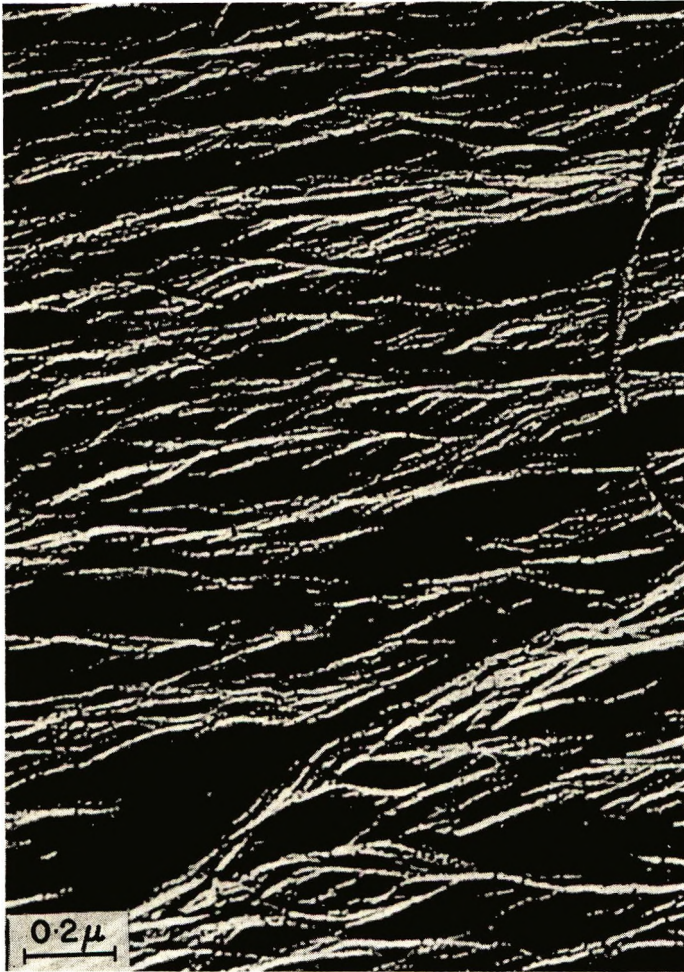
Fig. 12. Electron micrograph (negative print) showing the surface of a spruce wood fiber. The finest filaments show an axial texture similar to that observed in negatively stained preparations. The fibers were freeze-dried and replicated as described by Norberg. 29 Platinum shadowed at 30^\circ , magnification 60,000\times .
