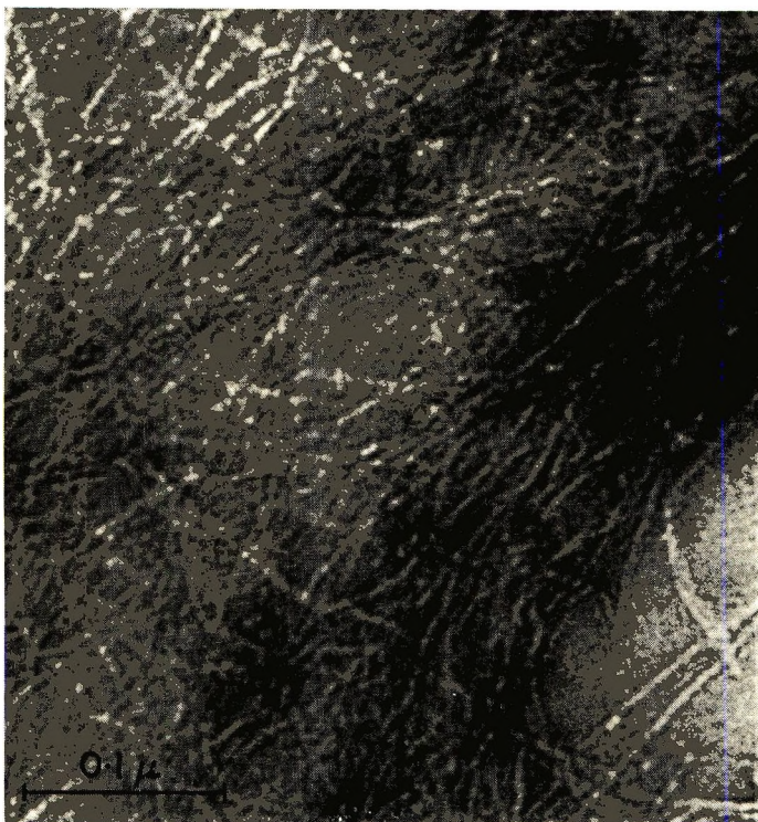
Fig. 5. Filamentary structure elements of Valonia microfibrils isolated by swelling and subsequent sonication. Negatively stained with uranyl acetate, magnification 240,000 \times .
