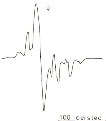
Fig. 10. Radicals II and XI in combination in vacuo at room temperature immediately after 1 Mrad electron irradiation in air, this dose being sufficiently high for all the dissolved oxygen to be exhausted.
