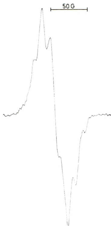
Fig. 7. \Delta M_S = 2 transition in a powdered MA crystal. Microwave power 25 mW, modulation amplitude 4 G.
