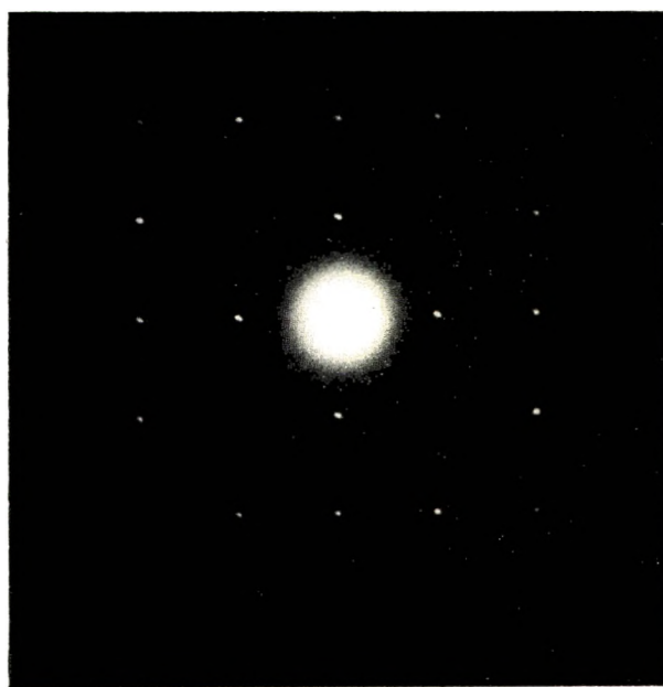
Fig. 3. Electron diffraction pattern from single crystals of amylose- \alpha -naphthol complex.
