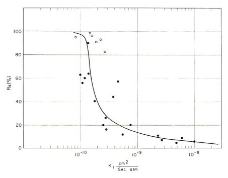
Fig. 4. Relationship between salt rejection  $R_s$  in reverse osmosis and log  $K_1$  for nonionic polymer membranes: (O) cellulose acetate membranes, Eastman E-398-3, cast from various solvents; (——) values calculated from eq. (16) for the model case.
