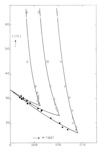
Fig. 7. Loci of the maxima of A and B for the three polystyrene samples in cyclohexane:  $(\bigcirc)$  maximum of A,  $(\bullet)$  maximum of B (sample 7a);  $(\Box)$  maximum of A,  $(\bullet)$  maximum of B (sample 1a);  $(\triangle)$  maximum of A,  $(\blacktriangle)$  maximum of B (sample 5a).
