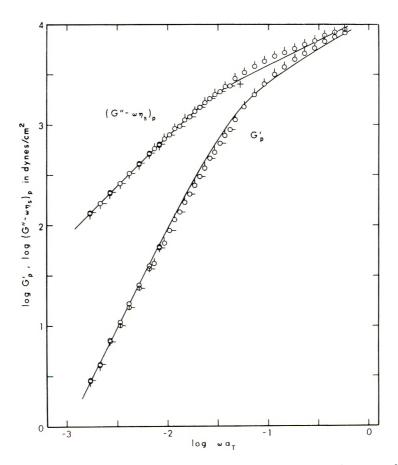
Fig. 2. Logarithmic plots of  $G'_p$  and  $(G''-\omega\eta_s)_p$  against  $\omega a_T$  for  $4''_{0}$  polystyrene, M = 394,000 in Aroclor 1260, reduced to  $35^{\circ}$ C: ( $\circlearrowright$ ) measured at  $45^{\circ}$ C: ( $\bigcirc_7 \circ$ ) measured at  $58^{\circ}$ C. Curves represent Rouse theory with origin of dimensionless plot at cross.
