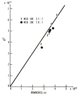
Fig. 9. Plots of chains/cc. vs. branches/cc in polyurethane.
