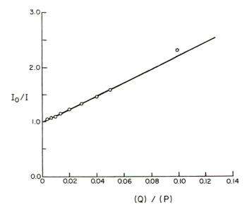
Fig. 7. Determination of the Stern-Volmer constant for the self-quenching of quinine from data in PVS solution.
