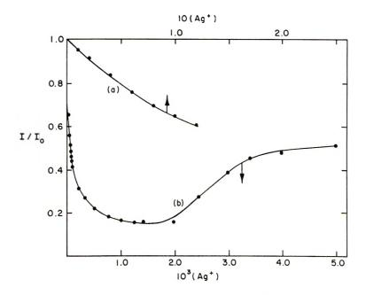
Fig. 4. Effect of PVS on the quenching of quinine fluorescence by Ag<sup>+</sup>: (a) no PVS; (b)  $3 \times 10^{-4} N$  PVS.
