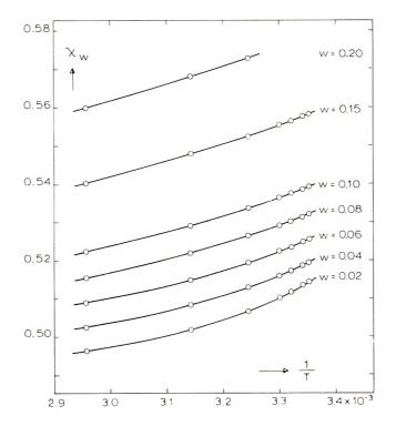
Fig. 2. Interaction parameter  $\chi_w$  vs. 1/T for solutions of polystyrene 1a ( $M_w = 163000$ ) in cyclohexane.
