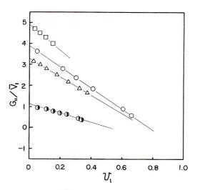
Fig. 6. Clustering function  $G_{11}/\overline{V}_1$  vs.  $v_1$  in the system polypropylene–CCl<sub>4</sub> at 25 °C: ( $\bigcirc$ ) atactic polypropylene; ( $\bigcirc$ ) isotactic polypropylene; ( $\square$ ) polyethylene–methyl bromide;<sup>6</sup> ( $\triangle$ ) polyethylene–ethyl bromide.<sup>6</sup>
