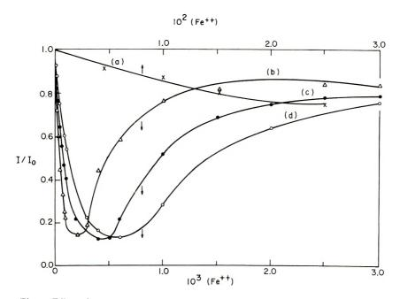
Fig. 3. Effect of PVS on the quenching of quinine fluorescence by Fe<sup>++</sup> in the presence of  $10^{-3} M$  HClO<sub>4</sub>: (a) no PVS; (b)  $10^{-3} N$  PVS; (c)  $2 \times 10^{-3} N$  PVS; (d)  $3 \times 10^{-3} N$  PVS.
