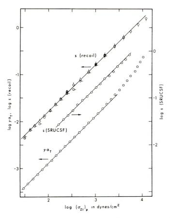
Fig. 4. Logarithmic plot of s from recoil, s from SRUCSF, and  $\dot{\gamma}a_T$  against shear stress reduced to 35°C; replicate measurements of s from recoil at 35°C indicated by different pip positions. Lines are drawn with unit slope.
