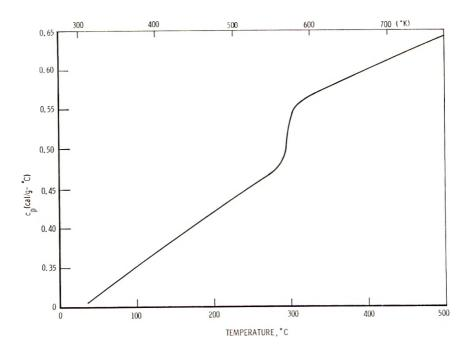
Fig. 6. Plot of heat capacity vs. temperature for polymer 14.
