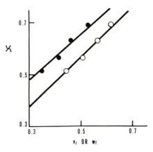
Fig. 6. Variation of interaction parameter with  $(\bigcirc)$  volume fraction of polymer in swollen polyurethane and with  $(\bullet)$  weight fraction of HMDI in polyurethane (series A).
