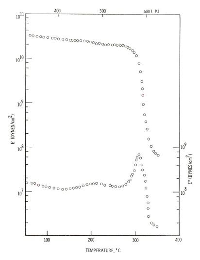
Fig. 8. Plot of dynamic tensile modulus E' and storage modulus E'' vs. temperature (measurements made at a heating rate of 5°C/min in a helium atmosphere, frequency 110 cps).
