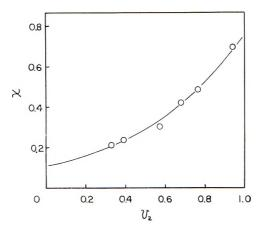
Fig. 2. Interaction parameter  $\mathbf{x}$  vs.  $v_2$  for the system atactic polypropylene-CCl<sub>4</sub> at 25°C:  $(--\cdot) \mathbf{x} = 0.113 \exp \{1.879 v_2\}$ .
