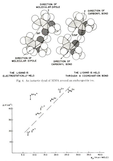
Fig. 5.  $\Delta \overline{\nu}$  vs. the calculated value of the electrostatic interaction potential  $\Phi_p$  (in kcal/mole) for MA.
