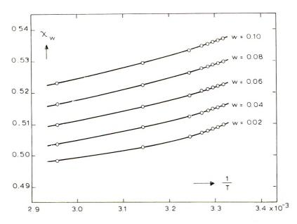
Fig. 3. Interaction parameter  $\chi_w$  vs. 1/T for solutions of polystyrene 5a ( $M_w = 520000$ ) in cyclohexane.
