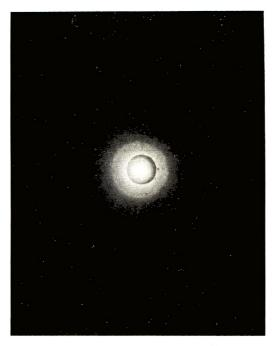
Fig. 3. Flat-plate x-ray photograph of polymer 14 at  $25^{\circ}$ C. Nickel-filtered CuK  $\alpha$  radiation, specimen-to-film distance 5 cm.
