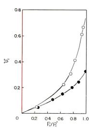
Fig. 1. Sorption isotherms of carbon tetrachloride in polypropylene at  $25^{\circ}$ C: (O) atactic polypropylene; ( $\bullet$ ) isotactic polypropylene.
