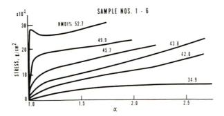
Fig. 1. Stress vs. extension ratio  $\alpha$  in dry (unswollen) polyurethane (series A) films, NCO:OH = 2.1:1.
