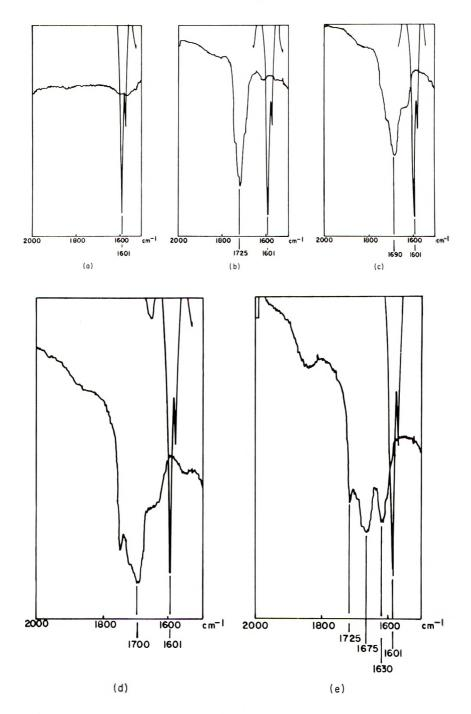
Fig. 3. Infrared spectra in the vicinity of the C=O stretching frequency:  $(a) \operatorname{Zn}^{2+}$  montmorillonite;  $(b) \operatorname{Cs}^+$  montmorillonite-methyl acetate complex;  $(c) \operatorname{Ca}^{2+}$  montmorillonite-methyl acetate complex;  $(d) \operatorname{Zn}^{2+}$  montmorillonite-methyl acetate complex;  $(e) \operatorname{Zn}^{2+}$  montmorillonite-MMA complex.
