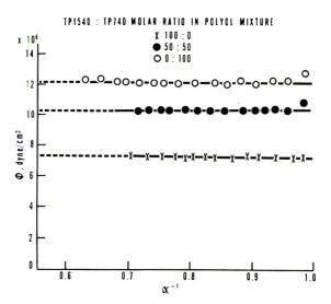
Fig. 4. Plots of  $\phi$  vs.  $\alpha^{-1}$  for polyurethane thin films swollen in benzene.
