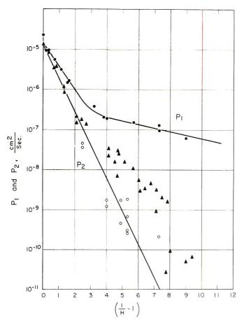
Fig. 2. Dependence of  $P_1$  (diffusive permeability of water) and  $P_2$  (diffusive permeability of NaCl) on (1-H)/H: (O) data of Lonsdale et al.;<sup>9</sup> ( $\Delta$ ) data of Yasuda et al.;<sup>6</sup> ( $\bullet$ ) data of Yasuda et al.<sup>1</sup>
