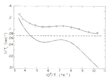
Fig. 2. Separation procedure used to extract  $(1/T_1)_{\text{corr}}$  illustrated for sample PS 2  $(\overline{M}_n = 41,500)$ . With the background relaxation (--) adjusted to 0.07 sec<sup>-1</sup>, the remaining relaxation curve (---) has a low temperature slope corresponding to 1.3 kcal/mole.
