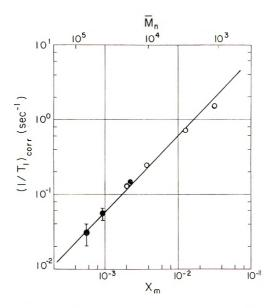
Fig. 3. Dependence of the corrected relaxation strength  $(1/T_1)_{\text{corr}}$  on the fraction of methyl protons  $X_m$  (•) for atactic polystyrene: also included are (O) the data of Connor<sup>1</sup> adjusted to 38 MHz.
