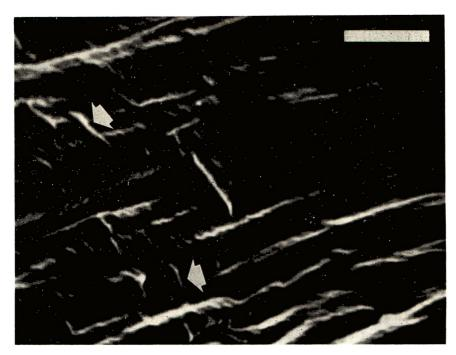
Fig. 4. Outer-sheath texture. Scanning electron micrograph; bar,  $1 \mu$ .
