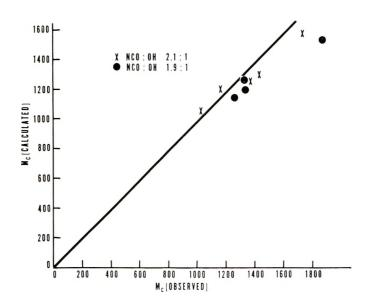
Fig. 10. Calculated and observed average molecular weight of chains between crosslinks.
