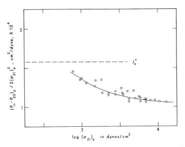
Fig. 6. Plot of  $(P_{11}-P_{22})_p/2(\sigma_{21})_p^2$  against logarithm of the shear stress. Horizontal line is the value of  $J_{\ell}^{\circ}$  over the indicated range from creep recovery measurements.
