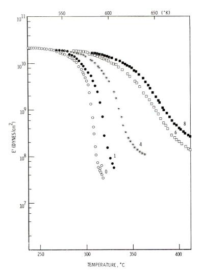
Fig. 9. Plot of dynamic storage modulus vs. temperature. Effect of thermal history on E' (thermal cycling for 1, 4, 6, and 8 hr in a helium atmosphere).
