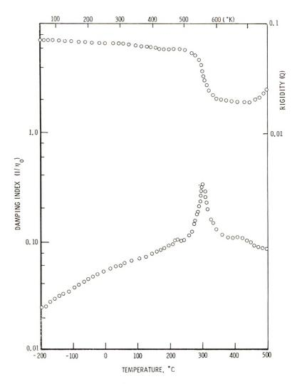
Fig. 11. Plot of damping and rigidity index vs. temperature (measurement made at a heating rate of  $5^{\circ}$ C/min in a helium atmosphere).
