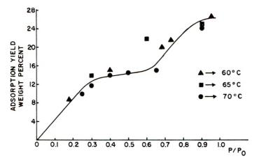
Fig. 2. Adsorption isotherm for Ca<sup>2+</sup> montmorillonite: (▲) 60°C; (■) 65°C; (●) 70°C.
