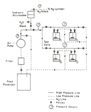
Fig. 1. Schematic drawing of the reverse osmosis test loop.
