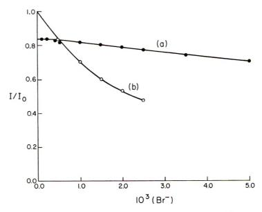
Fig. 5. Effect of PVS in the quenching of quinine fluorescence by Br<sup>-</sup>: (a)  $10^{-4} N$  PVS; (b) no PVS.
