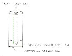
Fig. 3. Schematic diagram of strand indicating inner and outer sheaths discussed in the text.
