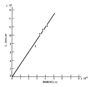
Fig. 5. Plot of  $C_1$  vs. branches/cc in polyurethane (series A).
