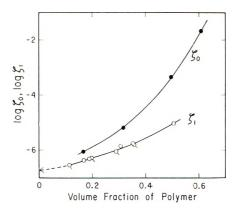
Fig. 1. Log  $\zeta_0$  and log  $\zeta_1$  plotted against  $v_2$  for samples Al (tagged circles) and A2 (circles without tags). Arrow on ordinate axis corresponds to glucose in pure solvent (value in water corrected to viscosity of diethylene glycol).
