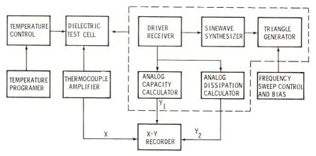
Fig. 1. Block diagram of dynamic scanning dielectrometer (Audrey II with high-tempperature test cell).
