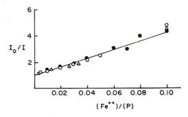
Fig. 6. Determination of  $C_{\text{eff}}^{\text{max}}$  from the dependence of the quinine fluorescence quenching on the [Fe<sup>++</sup>]/[P] ratio at various PVS concentrations: (•) 10<sup>-3</sup> N PVS; (O) 2 × 10<sup>-3</sup> N PVS; ( $\Delta$ ) 3 × 10<sup>-3</sup> N PVS.
