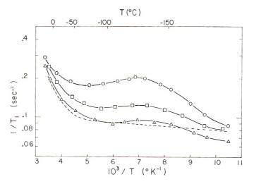
Fig. 1. Temperature dependence of the spin-lattice relaxation in atactic polystyrenes: (O)  $\overline{M}_n = 17,900$ ; (C)  $\overline{M}_n = 41,500$ ; ( $\Delta$ )  $\overline{M}_n = 67,400$ ; (--)  $\overline{M}_n = 780,000$ .
