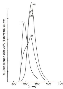
Fig. 1. Fluorescence of  $2 \times 10^{-5} M$  quinine solutions: (1) aqueous solutions; (2)  $10^{-4} M$ HClO<sub>4</sub>; (3)  $10^{-3} M$  HClO<sub>4</sub>; (4)  $10^{-1} M$  HClO<sub>4</sub>.
