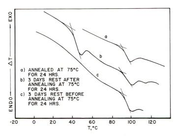
Fig. 4. Effect of annealing on nylon 11 transitions.
