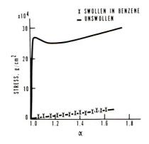
Fig. 3. Stress vs. extension ratio in dry and swollen polyurethane (sample 6).
