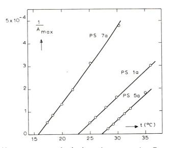
Fig. 12.  $1/A_{\text{max}}$  vs. temperature for the three polystyrene samples. Extrapolation to the temperature of the maximum of the spinodal.
