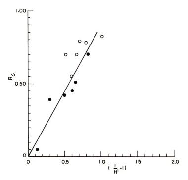
Fig. 3. Relationship between the salt rejection  $R_8$  and the parameter (1/H') - 1 for ionic polymer membranes: ( $\odot$ ) graft copolymer (PE-SSS), anionic; ( $\bullet$ ) block copolymer (ST-2VP), cationic. H' is the volume fraction of water in hydrophilic domain of membranes.
