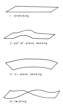
Fig. 14. Deformation in a ribbon segment.
