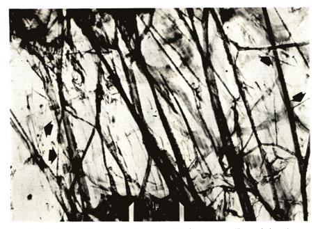
Fig. 8. Microtomed, Br<sub>2</sub>-stained section from the inner core. Transmission electron micrograph.
