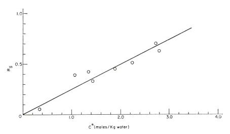
Fig. 2. Relationship between the salt rejection  $R_8$  and the fixed ion concentration  $C^*$  of the polystyrene-poly(2-vinylpyridine methyl bromide) block copolymer membranes.
