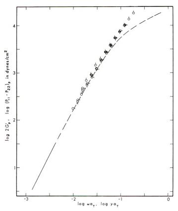
Fig. 3. Logarithmic plot of  $(P_{11}-P_{22})_p$  against  $\dot{\gamma}a_T$ , reduced to 35°C; replicate measurements at 58°C indicated by different pip positions. Curve represents data of Fig. 2 plotted as  $2G'_p$  against  $\omega a_T$ ; solid line indicates region with slope 2.
