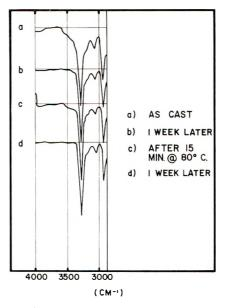
Fig. 5. Infrared spectra of nylon 6.
