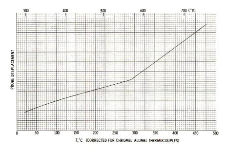
Fig. 7. Recorder trace of thermal expansion vs. temperature (heating rate 5°C/min, He atmosphere, displacement sensitivity  $1.35 \times 10^{-3}$  in./in. of chart paper).
