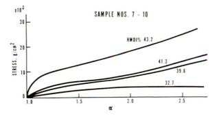
Fig. 2. Stress vs. extension ratio in dry (unswollen) polyurethane (series B) films, NCO:OH = 1.9:1.
