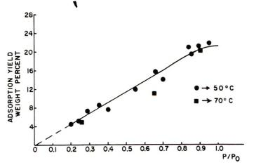
Fig. 1. Adsorption isotherm for Na<sup>+</sup> montmorillonite: (●) 50°C; (■) 70°C.
