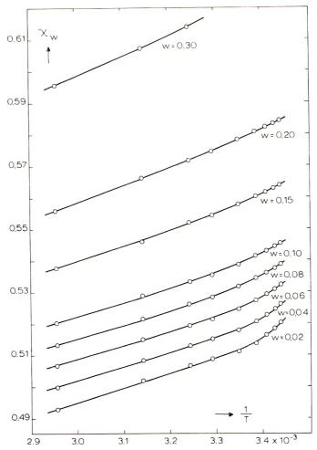
Fig. 1. Interaction parameter  $\chi_w$  vs. reciprocal temperature 1/T for solutions of polystyrene 7a ( $M_w = 51000$ ) in cyclohexane at various concentrations.
