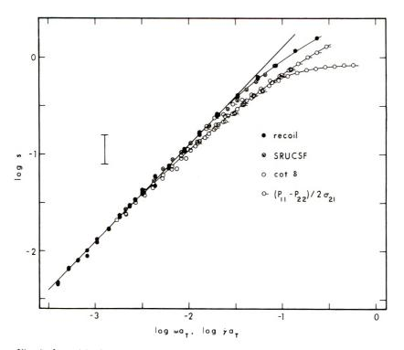
Fig. 5. Logarithmic plot of s from the indicated experiments against frequency or shear rate reduced to  $35^{\circ}$ C. Bold straight line drawn with unit slope. Vertical bar represents factor of 2.
