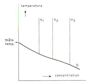
Fig. 4. Schematic plot showing concentrations where A and B pass through maxima as functions of temperature. Lines  $a_1$ ,  $a_2$ , and  $a_3$  correspond to maximum A for solutions of polymers with weight-average molecular weights increasing in order 1, 2, 3. Curve b locates maxima in B.
