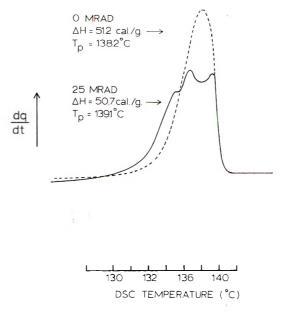
Fig. 11. Differential scanning calorimeter trace showing the effect of irradiation on the melting behavior of a transparent strand, produced at  $132^{\circ}$ C with a capillary of diameter 0.0762 cm and 1.0 cm/min plunger velocity.
