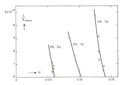
Fig. 13.  $1/A_{\text{max}}$  vs. concentration for the three polystyrene samples. Extrapolation to the concentration of the maximum of the spinodal.
