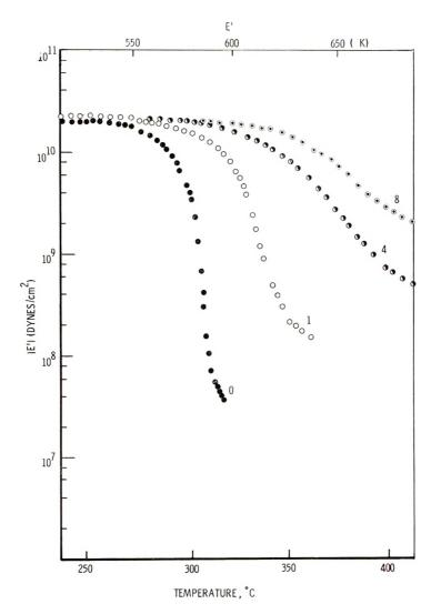
Fig. 10. Plot of dynamic storage modulus vs. temperature. Effect of thermal history on E' (thermal aging for 1, 4, and 8 hr in dry air).
