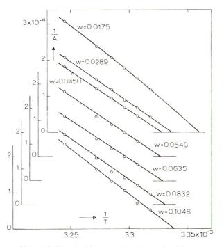
Fig. 10. Extrapolation of 1/A for sample 5a to spinodal temperatures.
