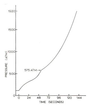
Fig. 1. Instron pressure trace at  $136^{\circ}$ C under a plunger velocity of 0.5 cm/min with a capillary of 0.0508 cm diameter, 1.55 cm length, and 90° entrance angle.
