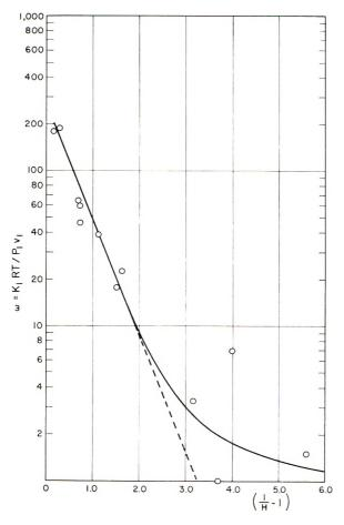
Fig. 3. Dependence of  $\omega = K_1 RT / v_1 P_1$  on (1-H)/H.
