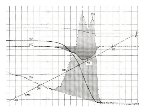
Fig. 4. Recorder trace of simultaneous TGA–DTA of 10 mg sample of polymer 14 (heating rate 5°C/min, TGA sensitivity 1.0 mg/in.; DTA sensitivity 10  $\mu$ V/in.; Pt–Pt 10 rd).
