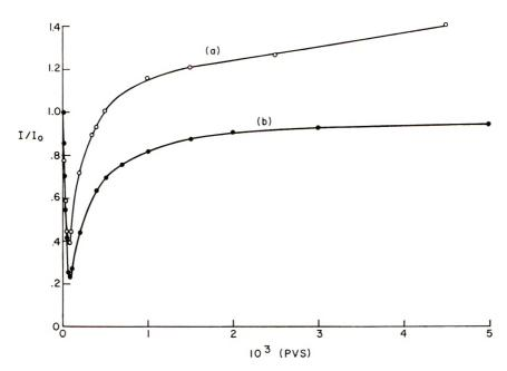
Fig. 2. Effect of poly(sodium vinylsulfonate) on the fluorescence intensities of quinine sulfate solutions: (a) fluorescence intensities at 462 nm, excitation at 400 nm; (b) fluorescence intensities at 452 nm, excitation at 346 nm.
