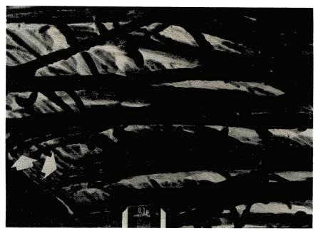
Fig. 7. Carbon replica showing inner core fiber bundles. Electron micrograph.
