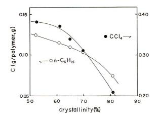
Fig. 5. Concentration of sorbed solvent vs. crystallinity in isotactic polypropylene at  $25^{\circ}$ C.
