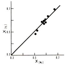
Fig. 7. Solvent-polymer interaction parameters derived from  $\chi = 0.077 + 0.97 v_t$ , [eq. (4a)] vs. solvent polymer-interaction parameters derived from  $\chi = 0.23 + 0.84 w_t$  [eq. (4b)].
