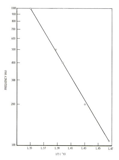
Fig. 13. Arrhenius plot for dielectric relaxation of polymer 14.
