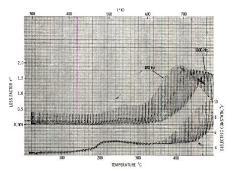
Fig. 12. Recorder trace of dissipation factor and capacitance vs. temperature (heating rate  $5^{\circ}$ C/min, He atmosphere, frequency sweeps 100 to 1000 Hz).
