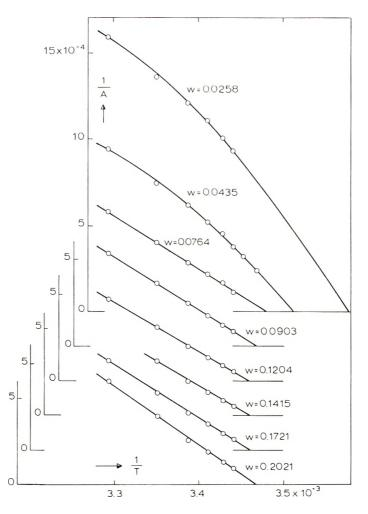
Fig. 8. Plots of 1/A vs. reciprocal temperature for sample 7a at various concentrations. Extrapolation to spinodal temperatures.
