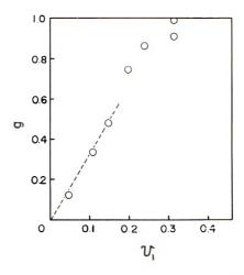
[Fig. 4. Values of g vs.  $v_1$  in isotactic polypropylene–CCl<sub>4</sub> at 25°C.
