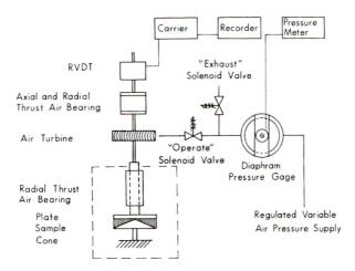
Fig. 1. Schematic representation of modification of the Weissenberg rheogoniometer for creep and recovery measurements.
