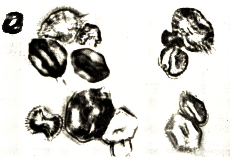
Fig. 8. Groups of axialite formed on slow cooling floating in the liquid. Photomicrograph, 750 \times .
