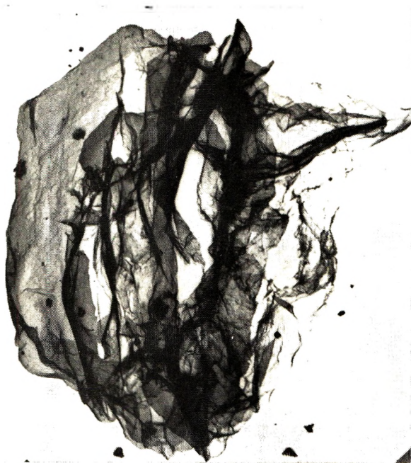
Fig. 15. Shaded transmission electron micrograph of an axialite formed at 85°C. Detachment replica, 3080 \times .
