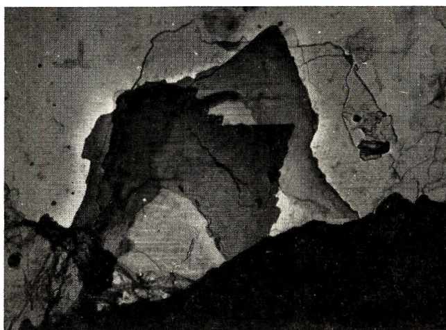
Fig. 17. Thick layer fragments. Unshadowed detachment replica, coated with carbon from different sides, with unequal intensity, electron micrograph, 8880 \times .
