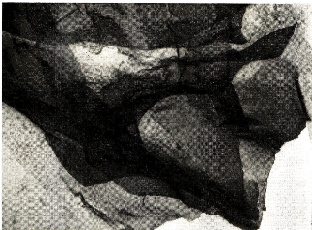
Fig. 19. Tip of an incipient axialite formed at 90°C. Shaded detachment replica, electron micrograph, 5698.×
