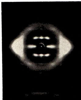
Fig. 3. Flat-plate x-ray diffraction pattern of nylon 8, \alpha -phase. Fiber axis vertical.
