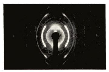
Fig. 4. Hexagonal POM. Spectrum at tilted fiber with  $CuK\alpha$  radiation.
