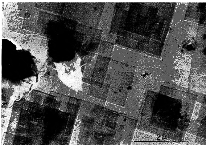
Fig. 6. Electron micrograph of a cellulose triacetate crystal showing (at the center of the photograph) the development of a closed sheet from two dislocations of opposite hand. Shadowed with gold-palladium. 11,400 \times .
