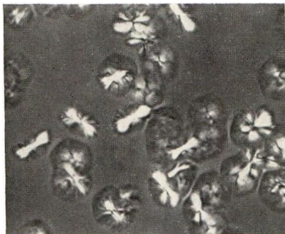
Fig. 13. Aggregates grown in isotactic polystyrene at 200°C. Note that hedritic aggregates seen obliquely appear as sheaflike objects. Phase contrast, \times 515 .
