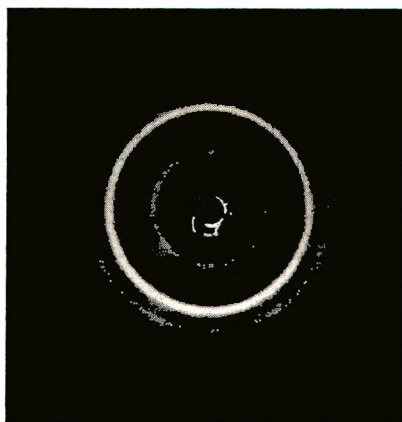
Fig. 12. X-ray diffraction pattern of hemicellulose of sulfate pulp from beech.
