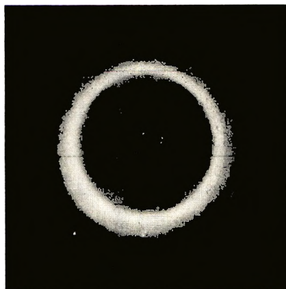
Fig. 10. X-ray diffraction pattern of xylan from beech having DP of 132.
