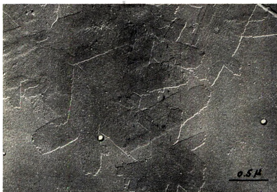
Fig. 11. Electron micrograph of solution growth crystals of VDC-VC copolymer (0.905 VDC). Crystallized in the form of a suspension from 0.015% monochlorobenzene solution, Pt shadowed, \times 30,000 .
