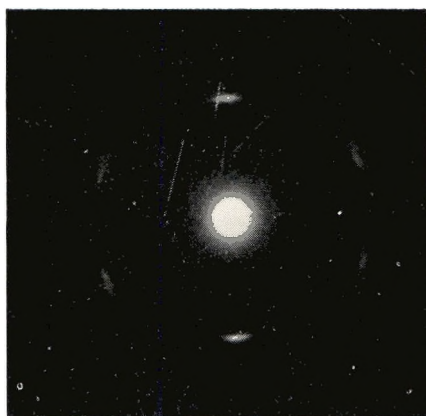
Fig. 5. Single crystal electron diffraction pattern given by Z-(\text{Cap})_{11}-\text{OH} from alcohol.
