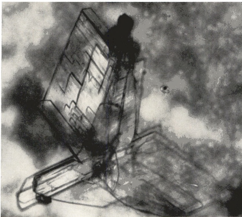
Fig. 2. Single crystals of Z-(\text{Cap})_{10}-\text{OH} grown from formic acid. Photomicrograph, 1000\times .
