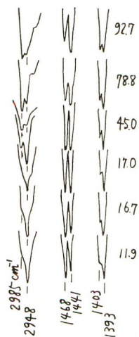
Fig. 6. The effect of composition in the monomer mixture on the infrared spectra of the copolymers in the region of 1400\text{--}3000\text{ cm}^{-1} . Numbers to the right of the figure indicate tetrafluoroethylene content of the monomer mixture (mole-%).
