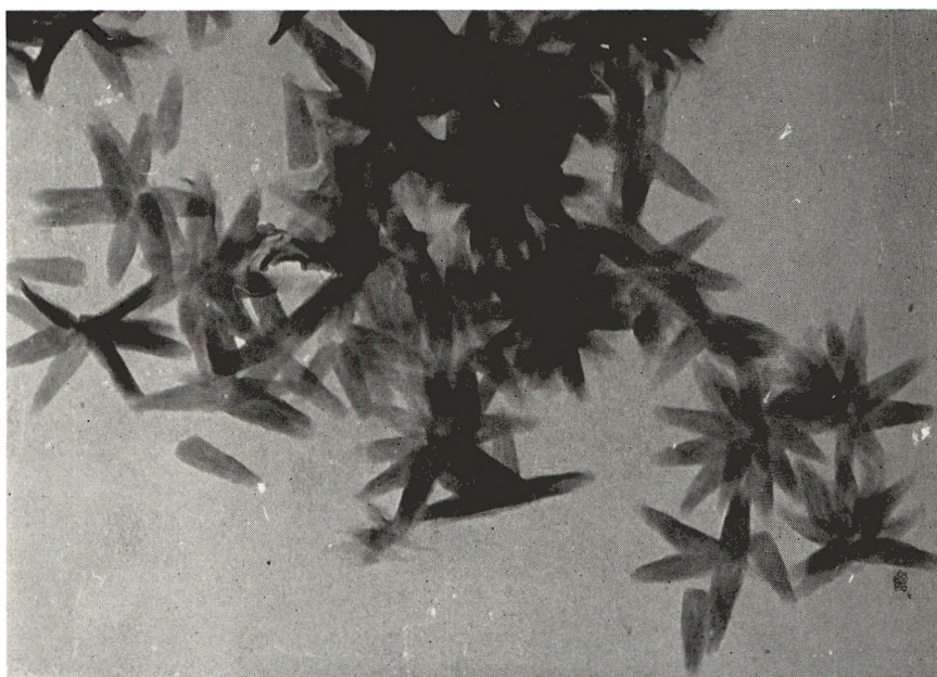
Fig. 3. Star-shaped aggregates of Z-(Cap) 11 -OH crystals from alcohol. Electron micrograph, 3000 \times .
