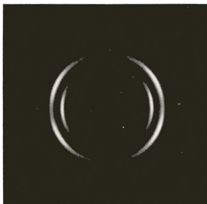
Fig. 3. X-ray diffraction pattern from sedimented mat of solution crystallized poly-(ethylene oxide) single crystals (high molecular weight Polyox resin). Mat normal, vertical in the present mounting, is perpendicular to the x-ray beam.
