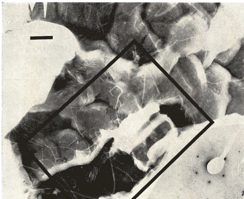
Fig. 8. Selected area diffraction pattern and corresponding bright field image of a Type III lamella in sample E. The area giving rise to the pattern is indicated on the micrograph, which is printed as a negative.
