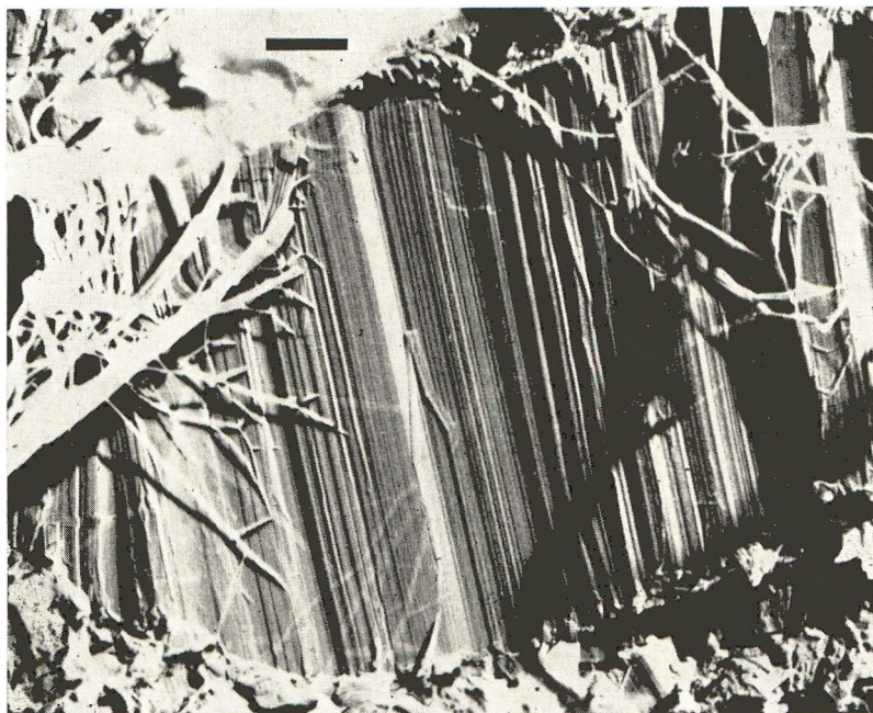
Fig. 5. Portion of the fracture surface of a large lamella in sample E. Several small kinks are present near the top center of the micrograph. This micrograph is printed as a negative.
