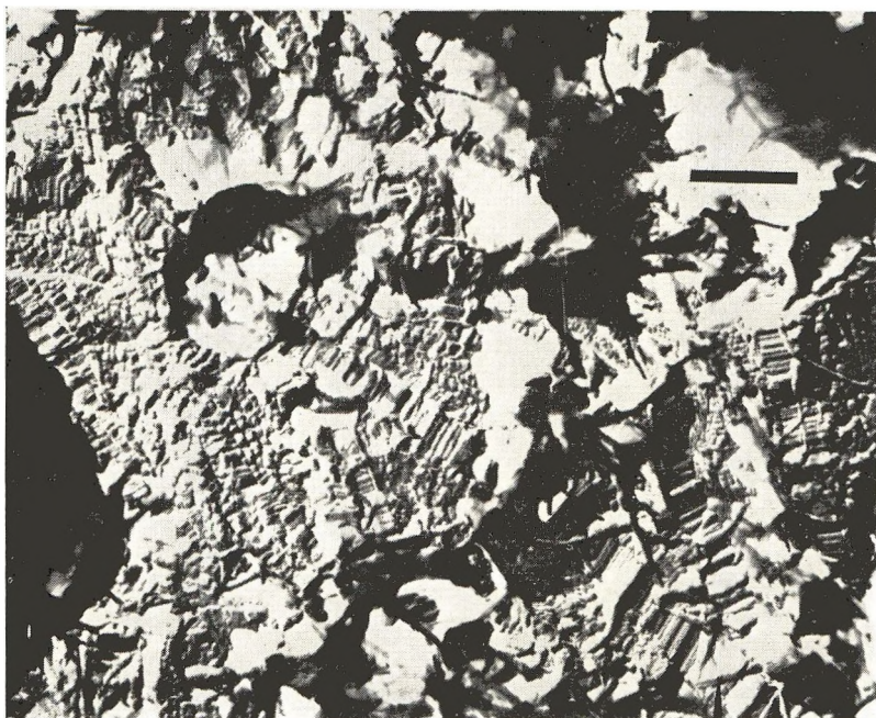
Fig. 2. Fracture surface of sample D. The dark areas in this and the other micrographs are a result of polyethylene adhering to the replica.
