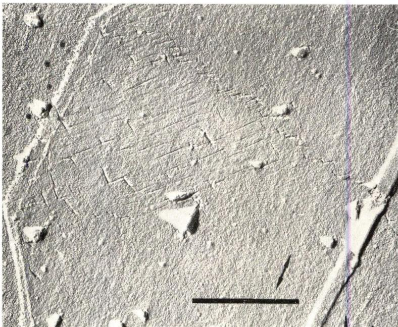
Fig. 7.  $\{100\}$  fold domain of a type E crystal which had been drawn  $50^\circ\text{C}$ . The pleat parallel to  $\mathbf{b}$  is on the right side of the figure.
