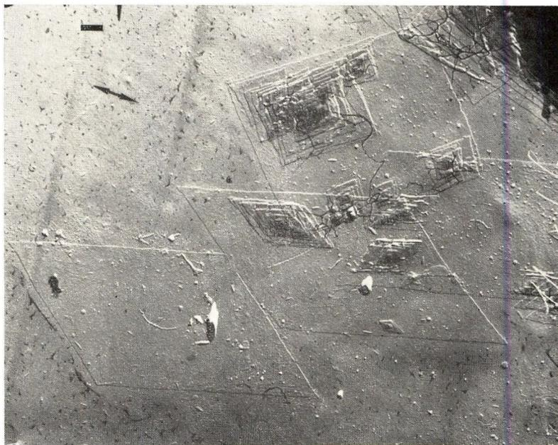
Fig. 1. Type A crystals drawn 25%. The draw direction is indicated by the arrows. The scale represents  $1 \mu$  and the shadowing angle is  $\tan^{-1} 2/8.5$  for all figures. The long fibers in the upper right were formed when the crystals were stripped from the Mylar.
