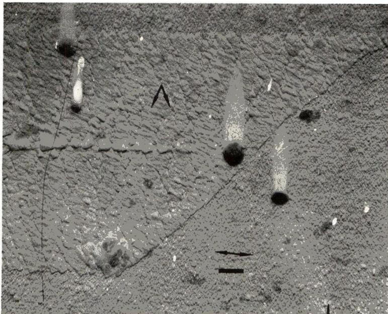
Fig. 5. Portion of a nylon 6 crystal drawn 100%. Two sets of cracks are present in the direction indicated by the single-headed arrows.
