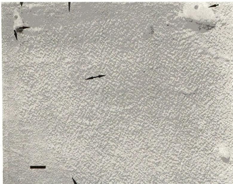
Fig. 8. Portion of a large polyoxymethylene crystal drawn 50%. The larger scale granulation corresponds to the crystal, the smaller to the Mylar. The crystal edges are indicated by the arrows.
