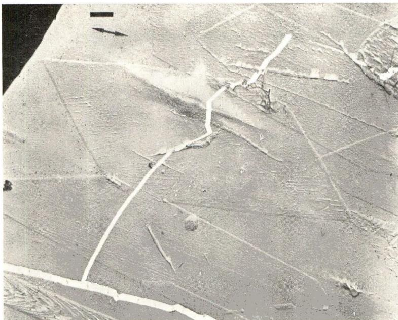
Fig. 8. Type E crystals drawn 150%. In the crystal on the bottom, the  $a$  axis is nearly parallel to the draw direction whereas in the crystal in the center it is almost normal to the draw direction.
