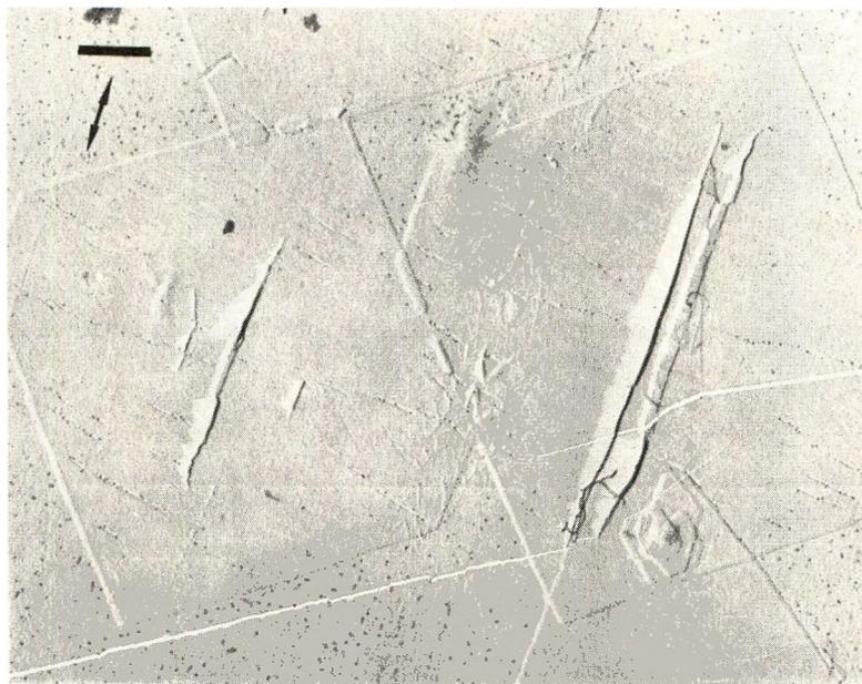
Fig. 6. Type E crystals drawn 25%. Note the Mylar fibers in the cracks and on the substrate.
