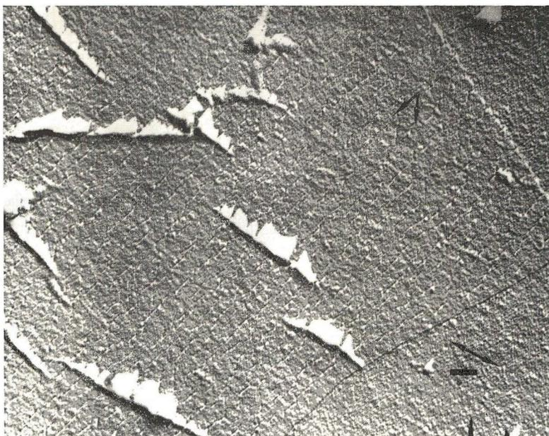
Fig. 7. Portion of a small star-shaped<sup>8</sup> polyoxymethylene crystal drawn 25%. Two sets of cracks can be observed, as indicated by the single-headed arrows.
