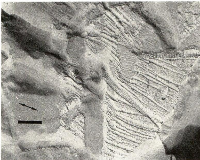
Fig. 3. Fibers drawn across an overgrowth crack and annealed at  $121^{\circ}\text{C}$ . for 1 hr. The substrate was drawn 100%.
