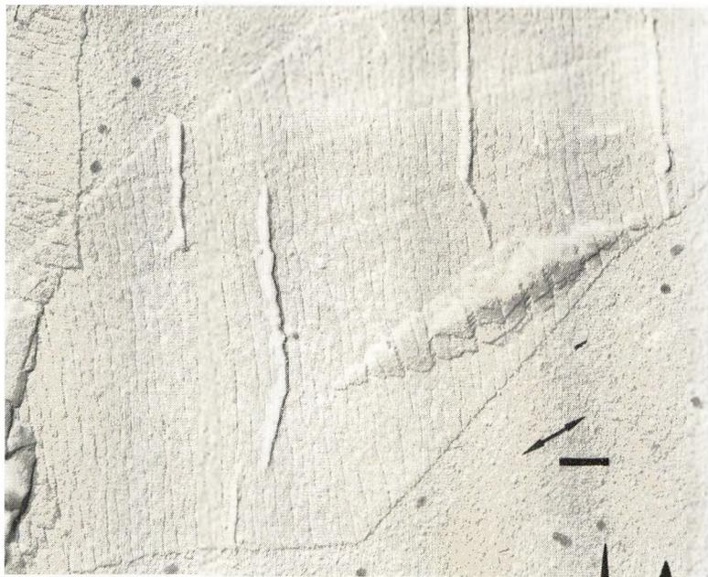
Fig. 2. Portion of a nylon 6 crystal drawn 25%. Fibers can be seen in the cracks on the overgrowth.
