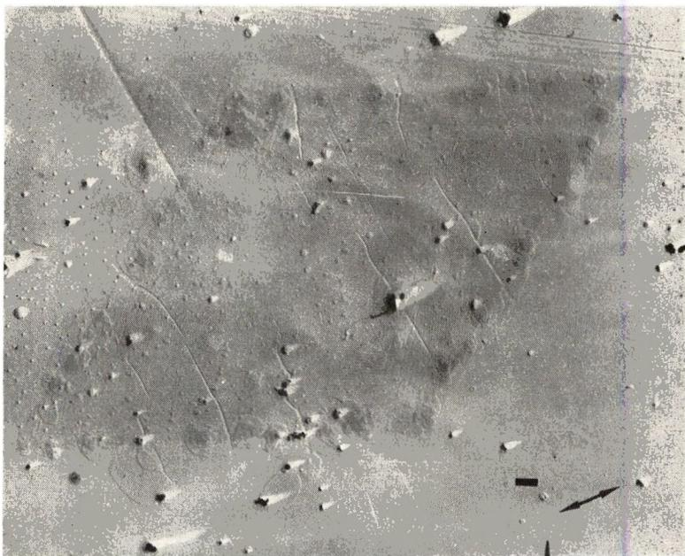
Fig. 3. Type C crystals drawn 10%. All of the overgrowths and thin edges are believed to have developed from low molecular weight polymer crystallizing during evaporation of the solvent. Fine corrugations resulting from collapse of the crystal during solvent removal can be seen here and in Fig. 4.
