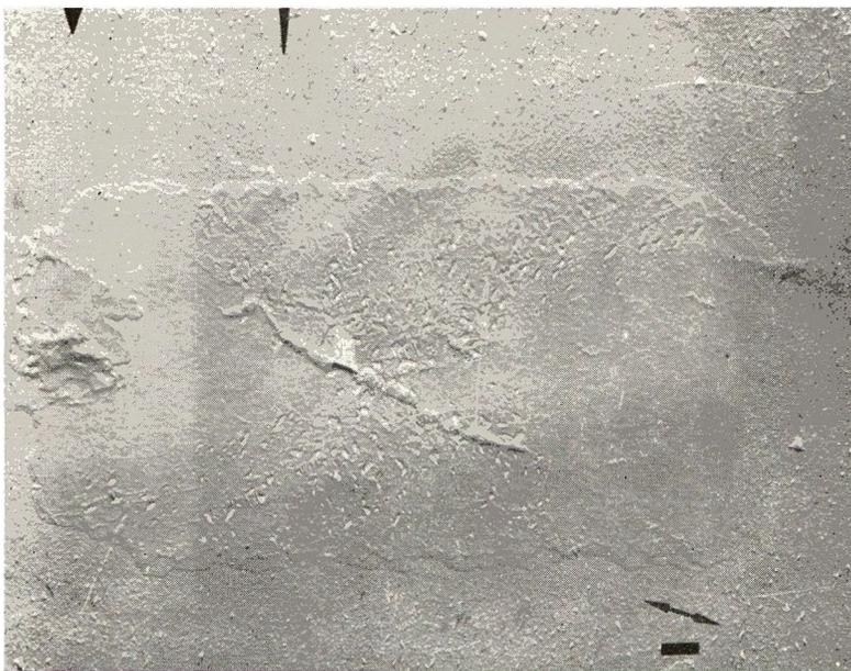
Fig. 9. Single crystal drawn 50% and annealed at 125°C. for 1 hr.
