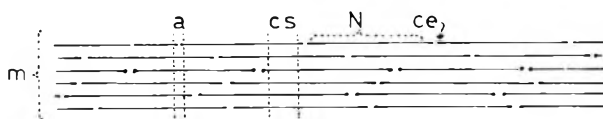
Fig. 2. Schematic model for the arrangement of cellulose molecules in an ideal cellulose microfibril: ( cs ) "continuous segment"; ( ce ) chain-ends; ( N ) length of a molecular chain; ( m ) number of molecules in cross section of a microfibril; ( a ) length of a segment dissolved around molecular chain-ends by initial acid hydrolysis.
