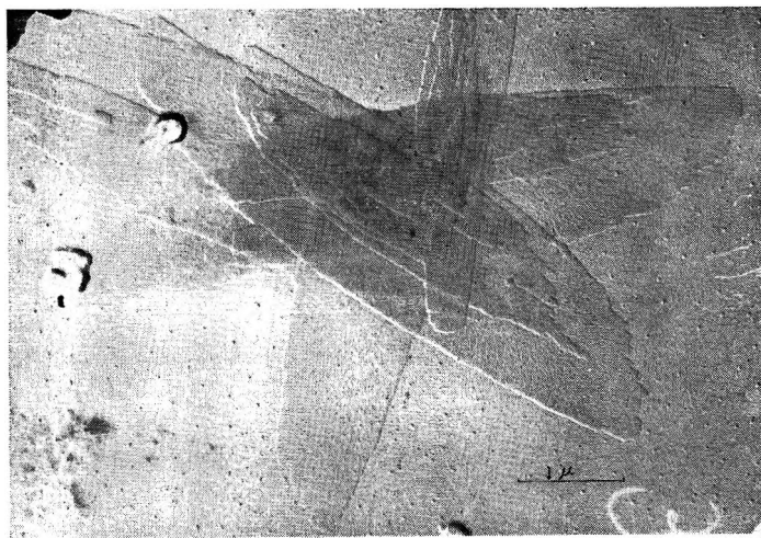
Fig. 12. Single crystals of poly(ethylene terephthalate) oligomer. The crystal shape is similar to that of PETP single crystals.
