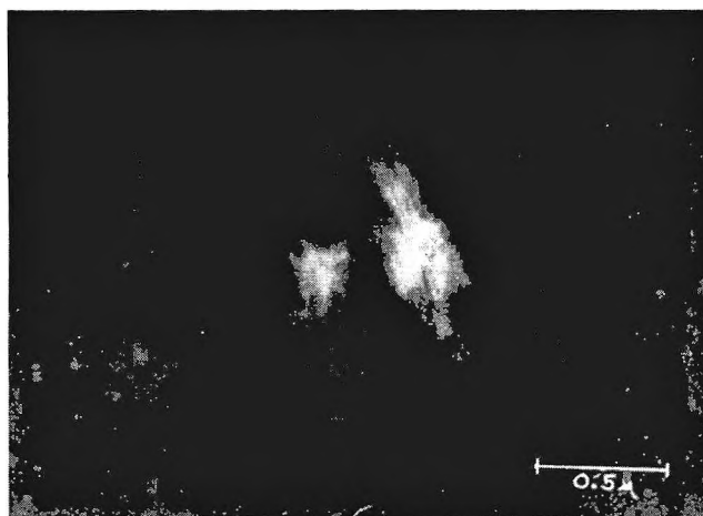
Fig. 7. Electron micrograph of undrawn nylon 66 longitudinal section including diametral sections of adjacent spherulites, filament axis horizontal.
