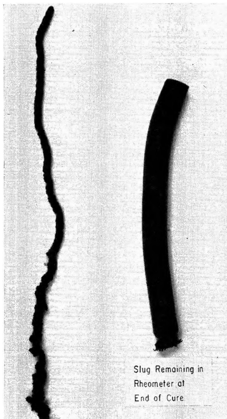
Fig. 27. Photograph of strand of EPR containing 50 pph of Philblack A carbon black extruded at 150°C.
