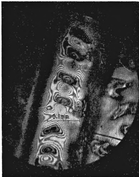
Fig. 4. Plexiglas II cleavage surface. Green light. Interference fringes from subsurface crazing.
