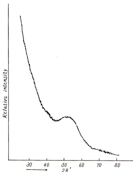
Fig. 5. Low-angle x-ray diffraction curve obtained on the film with the beam parallel to the film surface.
