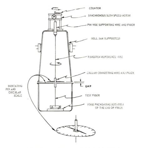
SKETCH OF APPARATUS USED FOR TORSION MEASUREMENTS BY THE DIRECT TWIST METHOD. SMALL SKETCH SHOWS DETAIL OF COLLAR WITH INDICATING PIN PASSING THROUGH CIRCULAR-MEASURING SCALE.
