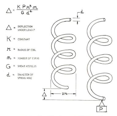
A MECHANICAL SPRING MODEL SHOWING THE VARIABLES INVOLVED IN THE EXTENSION OF A COIL UNDER LOAD.
