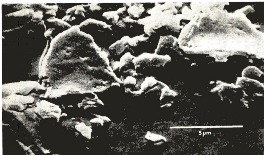
Figure 9. Scanning electron micrograph of the fragments produced after 2½ h shaking.
