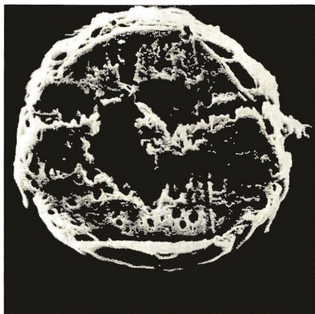
Figure 11. Cross section of a fragment from acid hydrolysis of fibers containing 119% PMMA
