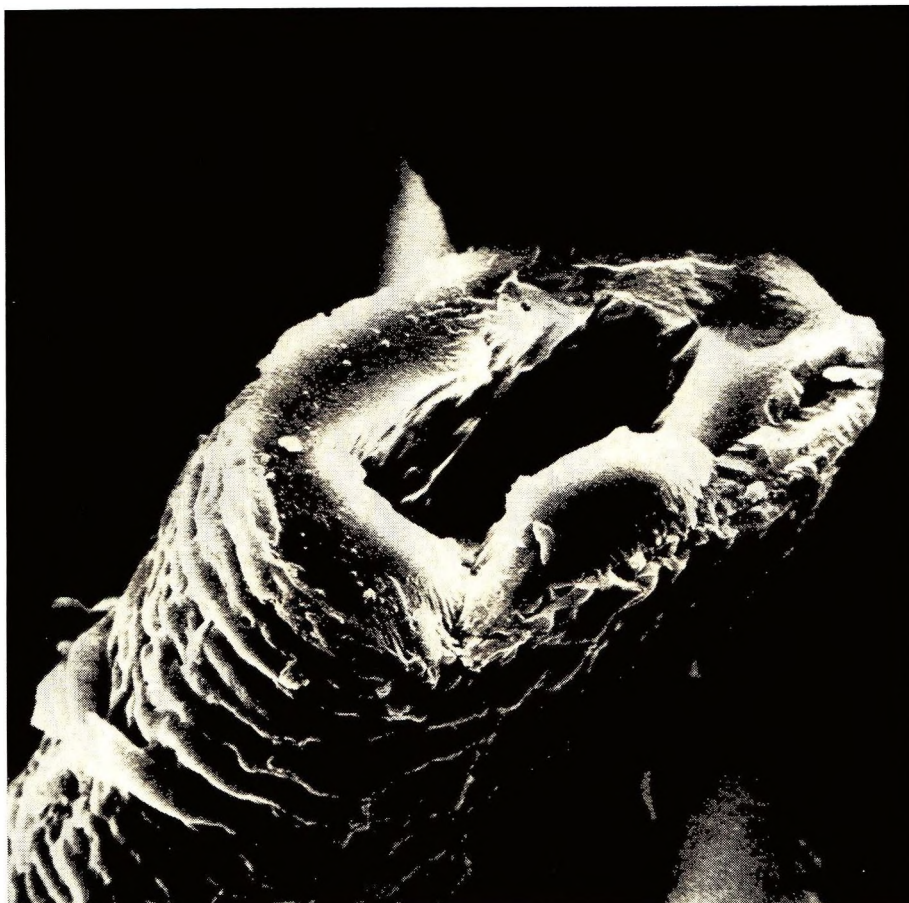
Figure 13. End view of a fragment from sodium sulfide reaction with hair fibers containing 119% PMMA add-on
