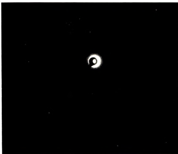
Figure 3. Typical small-angle diffraction pattern of surfactant, Sunsoft O-30B
