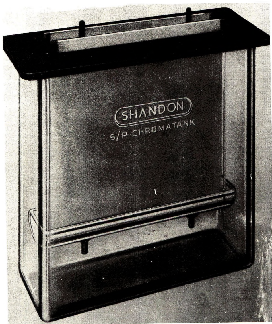
Figure 2. Apparatus for continuous elution TLC
