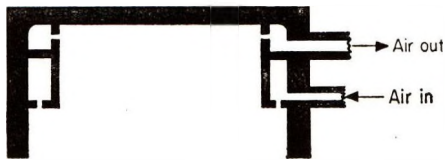
Figure 3. Hygrometric sweat measurement cell. The perspex cell directs air onto the sweating skin surface via a concentric ring of holes. The outgoing air has an elevated water content as a result of sweat evaporation.
