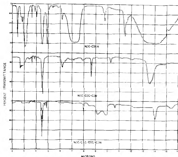
FIG. 2. INFRARED ABSORPTION SPECTRA OF MONOCYANOACETYLENE, DICYANOACETYLENE, AND DICYANODIACETYLENE.
