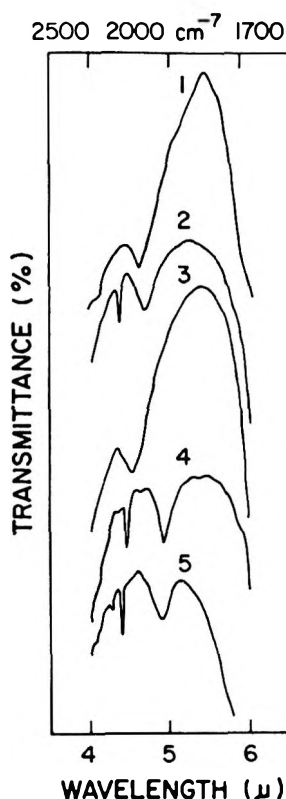
Figure 2.—Infrared spectra of \alpha - and \omega -cyanoamino acids in potassium bromide disks within 1700 and 2500 \text{cm}^{-1} ; (1) L - \gamma -cyano- \gamma -aminobutyric acid; (2) L - \gamma -cyano- \alpha -aminobutyric acid; (3) L - \beta -cyano- \beta -alanine; (4) L - \beta -cyanoalanine; (5) \alpha -cyanoglycine.
