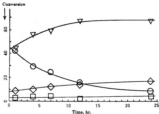
Figure 2.—Reaction of 1-iodoperfluoropropane and **3** at 70° (ref 4):  $CF_3CF_2CF_2I$ , 5.00 mmol; **3**, 10.00 mmol; ABN, 0.100 mmol.  $\nabla$ , trans  $C_b$ ;  $O$ , monoadduct A;  $\diamond$ , cis  $C_a$ ;  $\square$ , bis adduct B.
