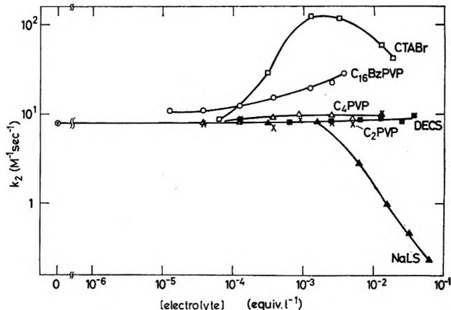
Figure 2.—Polyelectrolyte effect on the alkaline hydrolysis of PNPV at 30°: [PNPV] =  $5 \times 10^{-5}$  M; [NaOH] =  $2.5 \times 10^{-2}$  M.
