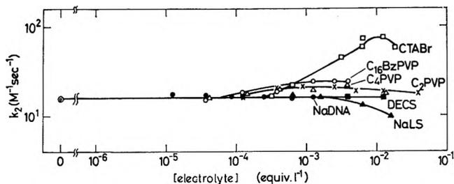
Figure 1.—Polyelectrolyte effect on the alkaline hydrolysis of PNPA at 30°: [PNPA] =  $5 \times 10^{-6}$  M, [NaOH] =  $2.5 \times 10^{-2}$  M.
