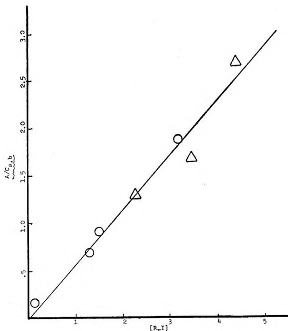
Figure 1.—Dependence of  $A/C_{a,b}$  on  $R_{F}I$  concentration:  $\Delta$ , mol/l. of  $CF_3CF_2CF_2I$  and **3**;  $O$ , **5**, **3**, and **6** (see Table I.)
