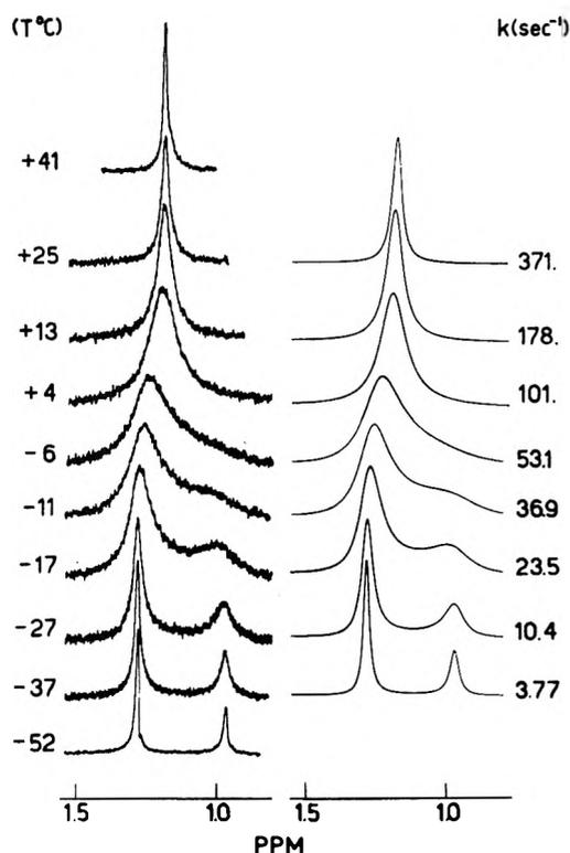
Figure 1.—Experimental (left) and computer-calculated (right) nmr spectra (90 MHz) of tri-*tert*-butylcyclopropenyl azide (0.08 *M*) in acetone-*d*<sub>6</sub> at various temperatures.
