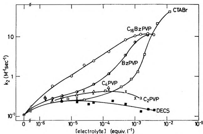
Figure 3.—Polyelectrolyte effect on the alkaline hydrolysis of PNPP at 30° in 30% ethanol-H<sub>2</sub>O: [PNPP] =  $4 \times 10^{-6}$  M, [NaOH] =  $10^{-3}$  M.
