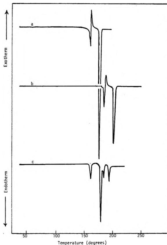
Figure 5.—Dsc of polymorphic glycosides: a, p -methoxyphenyl \beta -D-glucopyranoside; b, phenyl 2-acetamidotri- O -acetyl-2-deoxy- \beta -D-glucopyranoside; c, p -methoxyphenyl 2-acetamidotri- O -acetyl-2-deoxy- \beta -D-glucopyranoside.
