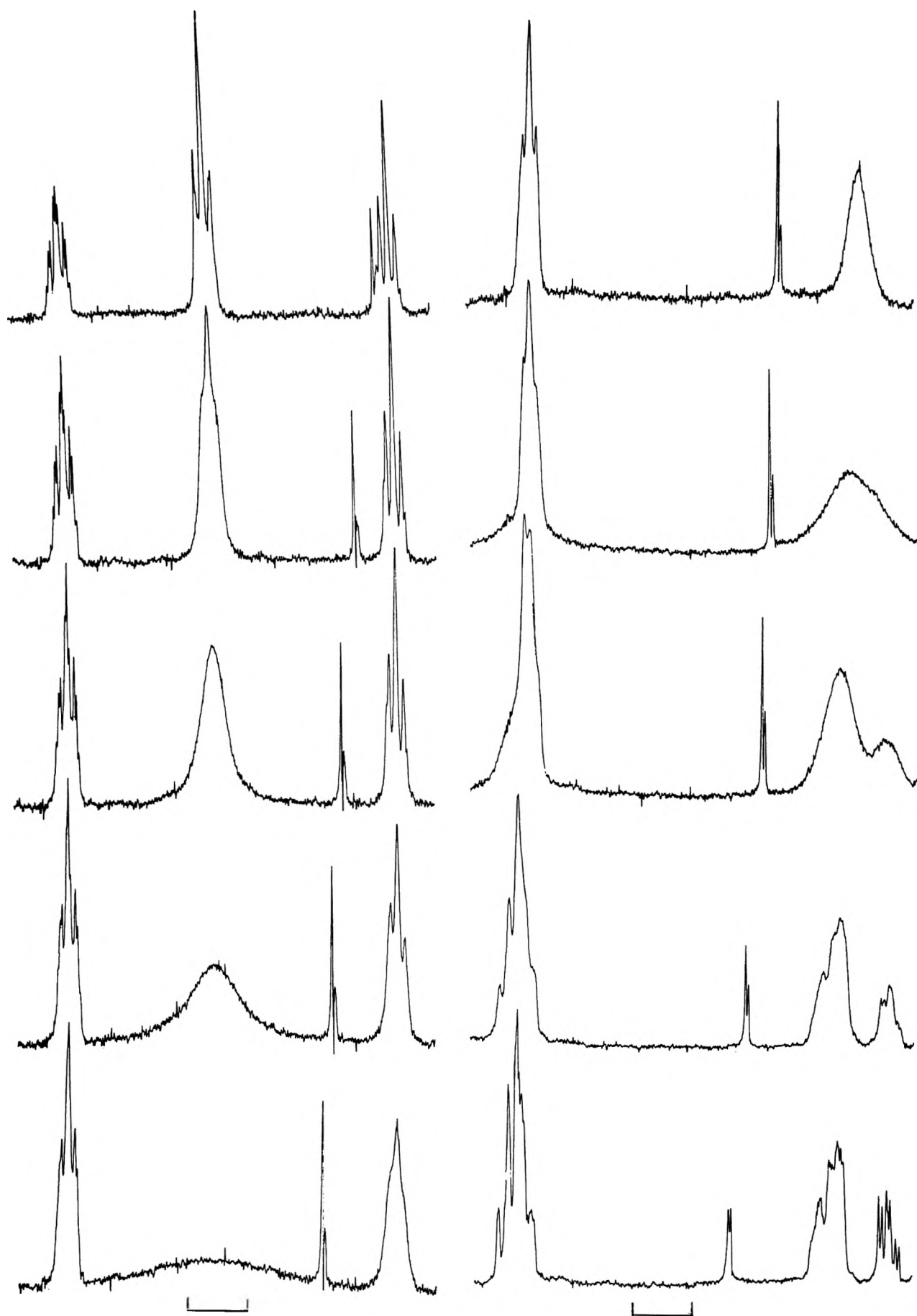
Figure 4.—The 90-MHz proton spectrum of barbaralone (1, X = C=O) in acetone- d_6 as a function of temperature: (left column from the top) 25, -0.5 , -14.5 , -26 , -35.5^\circ ; (right column from the top) -41 , -52 , -60 , -72 , -87.5^\circ . The calibration bar represents 50 Hz. The resonance positions at slow exchange are \delta 2.37 (t of d, H-1), 2.92 (m, H-2, H-8), 3.05 (m, H-5), 3.9 (d, impurity), 5.83 (br m, H-3, H-7), 5.95 (t, H-4, H-6).
