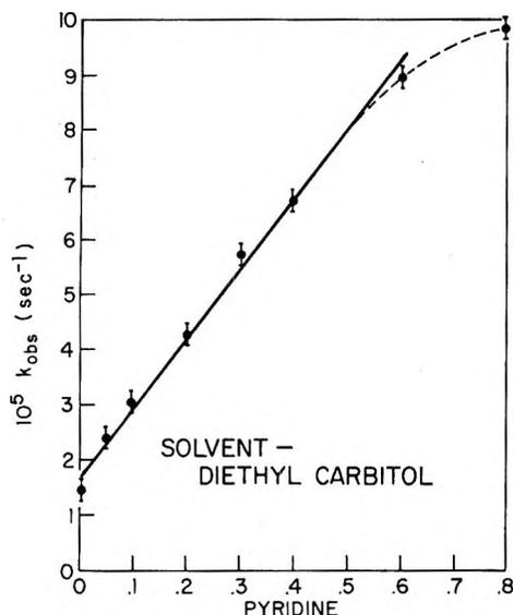
Figure 2. First-order kinetic behavior of allyl phenyl sulfide at 228.7° in the presence of various amounts of pyridine.
