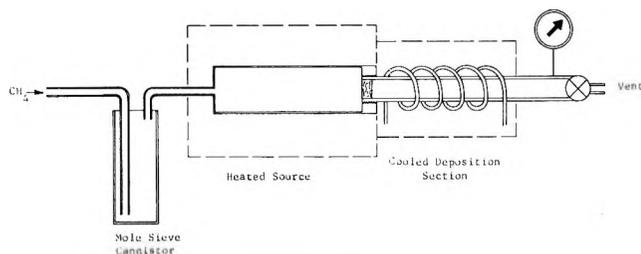
Figure 1. Schematic of clathrate formation apparatus.
