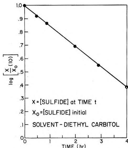
Figure 1. First-order kinetic behavior of allyl phenyl sulfide at 228.7° in the presence of an equimolar amount of pyridine (0.8 mol/l.).
