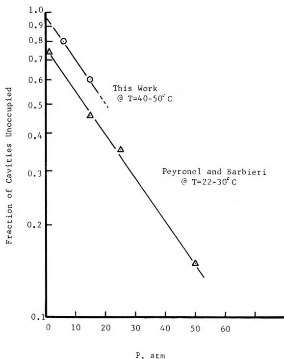
Figure 2. Pressure dependence of methane hydroquinone clathrate composition.
