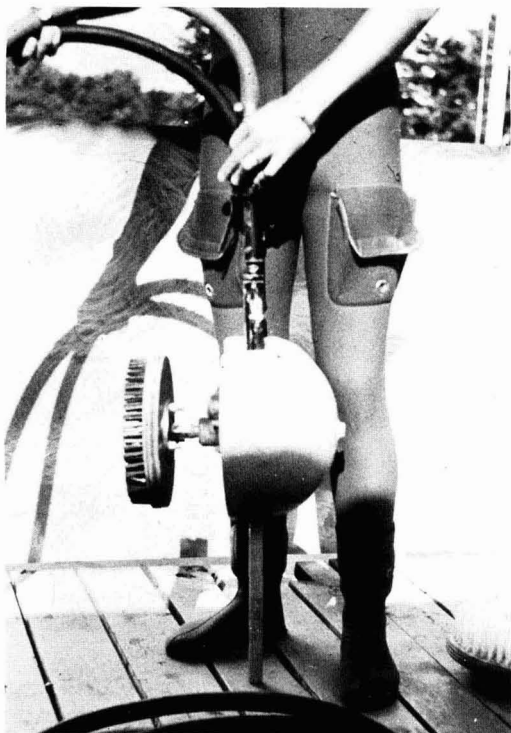
Figure 6—Diver controlled rotary brush assembly
