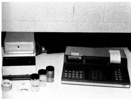
Figure 4—Equipment. The Hewlett-Packard HP9815A Calculator is shown here interfaced to a Mettler PL-200-02 Balance
