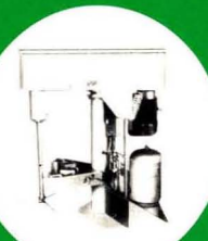
LOW-SPEED DISPENSERS "Bow Tie" blade provides intense shearing action for viscous products.
