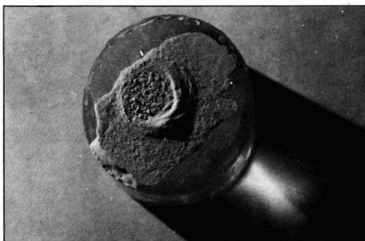
Figure 9—Typical cathodic delamination of sample
