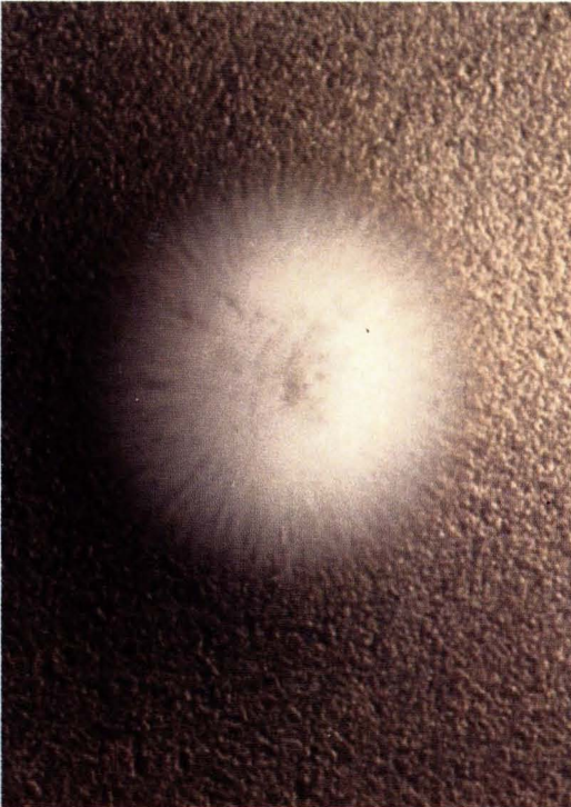
Coating with Hycar® RLP shows no damage after 10 lb. Gardner reverse impact test.
