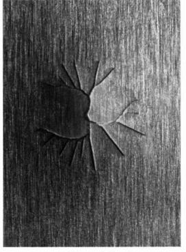
Coating without Hycar® RLP shows significant damage.
