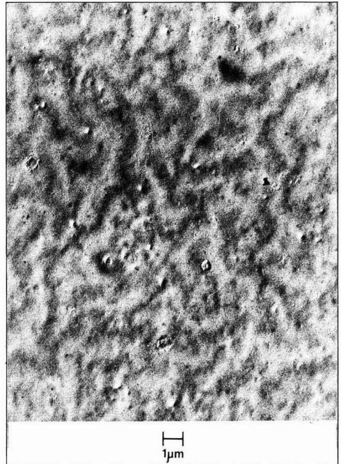
Figure 13—Electron micrograph of the surface (replica) of an acrylic water based coating containing 0.1% catalyst
