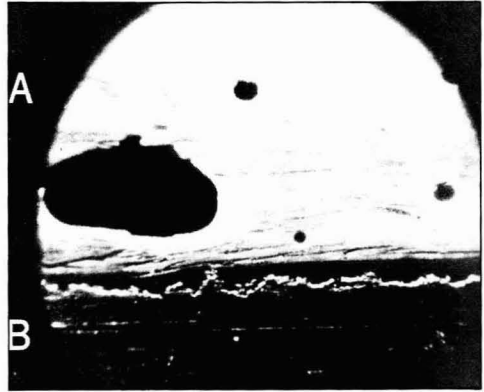
Figure 9—This trowel applied 125 mil polyester system shows delamination after 180 days test. 25X magnification also shows large void in the film. (A) Polyester laminate; (B) Steel
