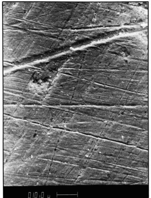
Figure 8—Typical surface of CRS panel wet abraded with 3-dimensional abrasive pad. SEM Magnification = 3000×
