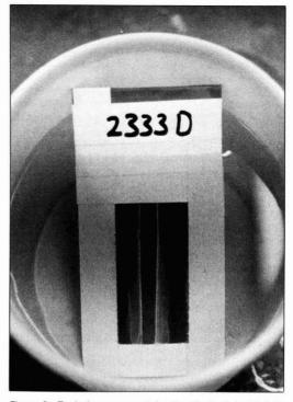
Figure 2—Typical arrangement for the 3% NaCl bullet hole immersion test. Each test vessel holds one panel only. Test solution is renewed after each seven days.
