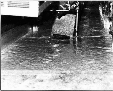
Figure 4—Cationic electrocoating of an air conditioner cabinet
